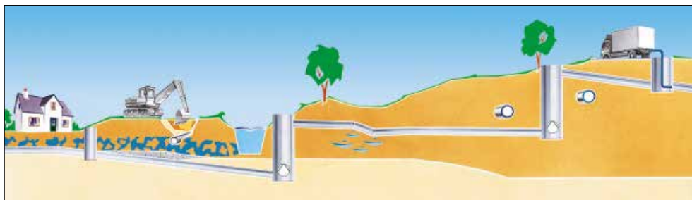
FIGURE 7 SCHEMATIC DRAWING OF A GRAVITY SEWER (SOURCE: ROEDIGER VAKUUM GMBH)
