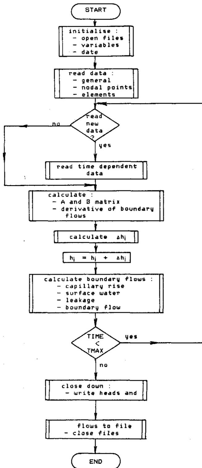
Figure 8 - Flow chart of program FEMSAT
