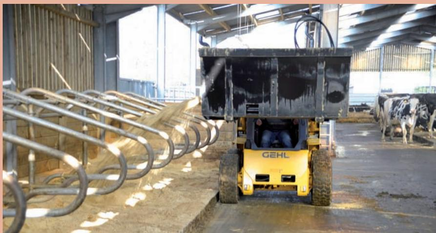
Side shooter: designed to spread sand – or sawdust – into cubicles
