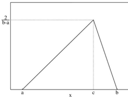
Figure YY: Example of a triangular distribution, where a and b are the minimum and maximum, and c the modal value. (source Wikipedia).
