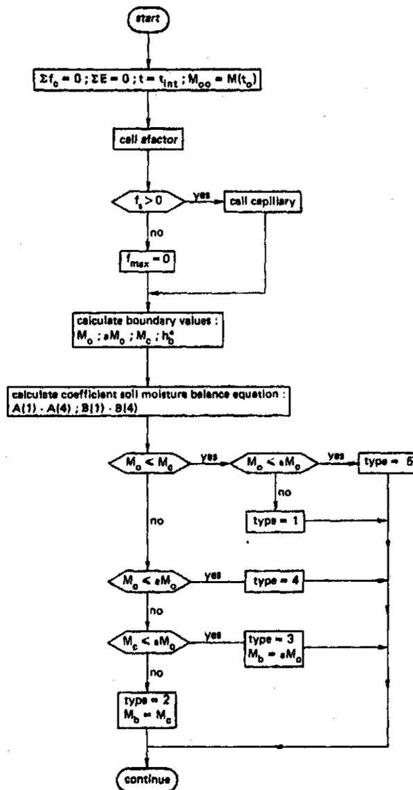
Fig. 10. Flow diagramme 'Initialization of constants' in subroutine 'EVA'
