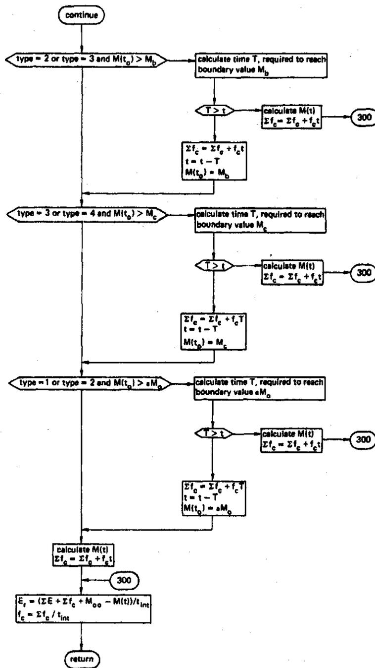
Fig. 12. Flow diagramme 'Evapotranspiration non-rice fields' of sub-routine 'EVA'
