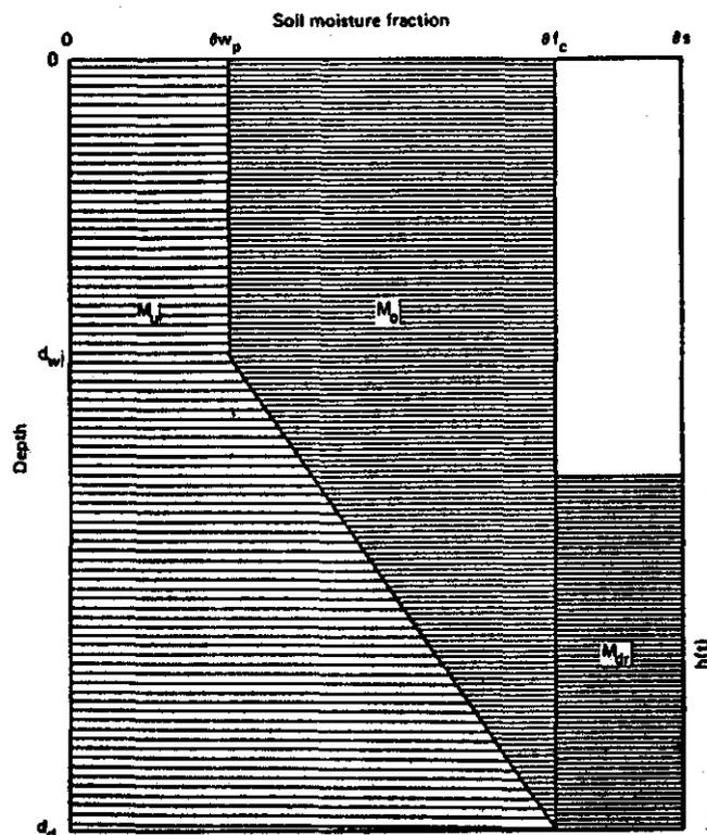
Fig. 1. Definition of unavailable moisture,  $M_u$  available moisture,  $M_o$  and drainable moisture,  $M_{dr}$
