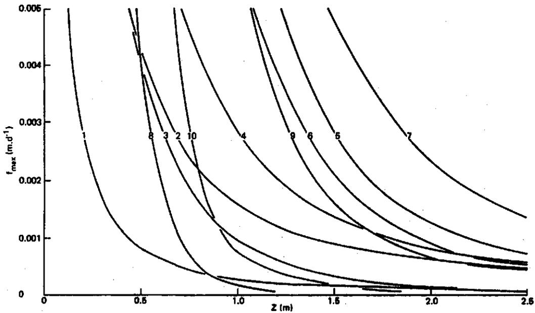
Fig. 3. Relation between maximum capillary flux  $f_{\max}$  ( $\text{m}\cdot\text{day}^{-1}$ ) and distance to groundwater table  $Z$  (m) assuming a soil moisture suction of 160 m for a number of standard soils (data from RIJTEMA, 1969)
