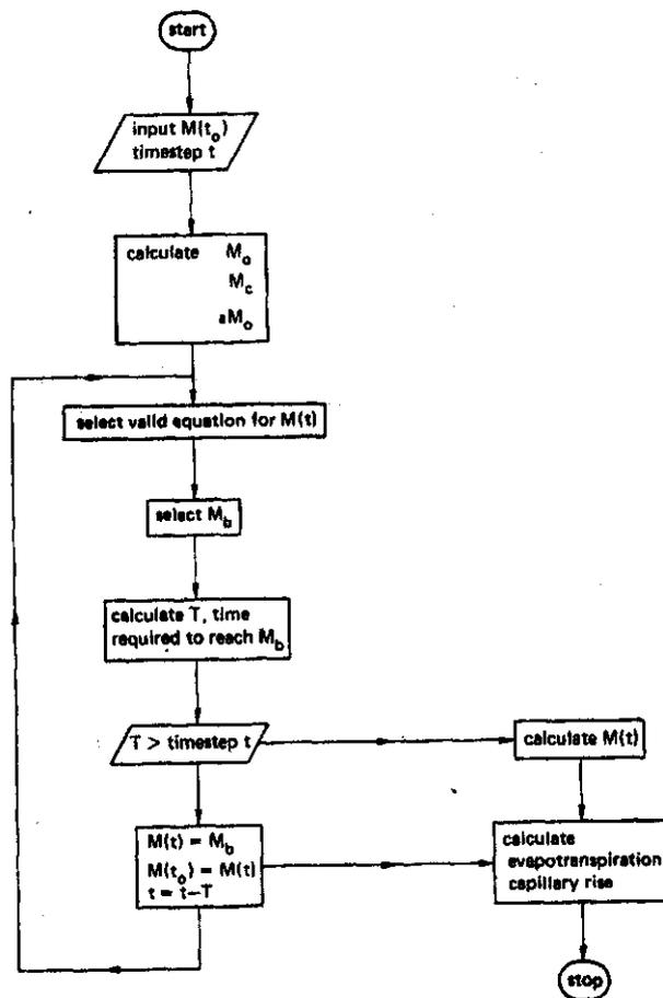
Fig. 2. Algorithm for the soil moisture balance
