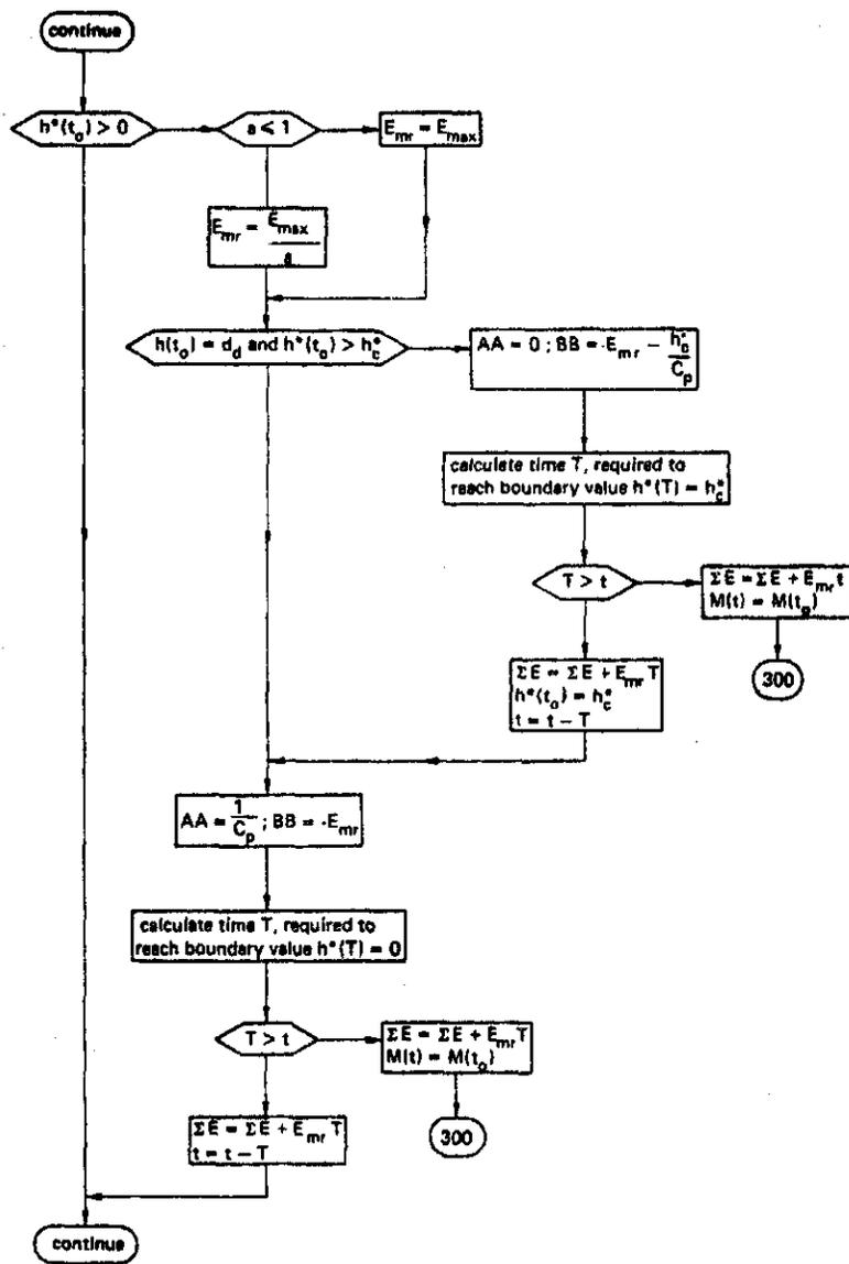
Fig. 11. Flow diagramme 'Evapotranspiration of rice fields' in sub-routine 'EVA'
