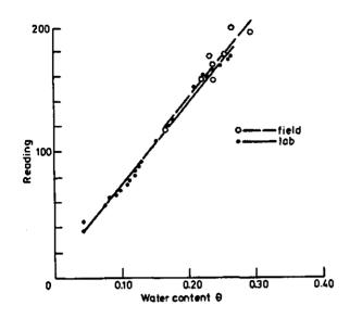
Figure 2. Calibration of the dielectric soil water content meter for the 'Sinderhoeve' experimental field at a depth of 10 cm below surface. The reading of the instrument is plotted against the gravimetrically-determined volumetric soil water content 0. The field calibration curve is the result of linear regression, the second order laboratory calibration curve of polynomial regression
