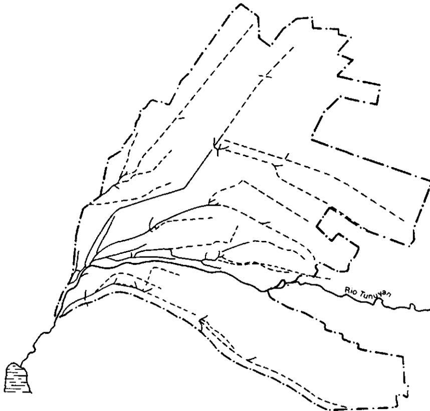
Fig 1.1 Lay out of Río Tunuyán Irrigation Scheme showing primary canals (—), secondary canals (----) and the boundary of the command area (-·-·-).
