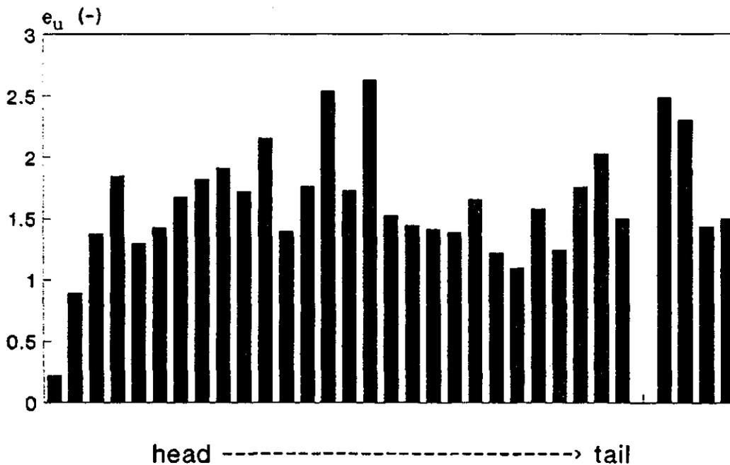
Fig 4.3 Tertiary unit efficiency ( $e_u(i,j)$ ) for all tertiary units of the Viejo Retamo in January regarding the supply of surface water.
