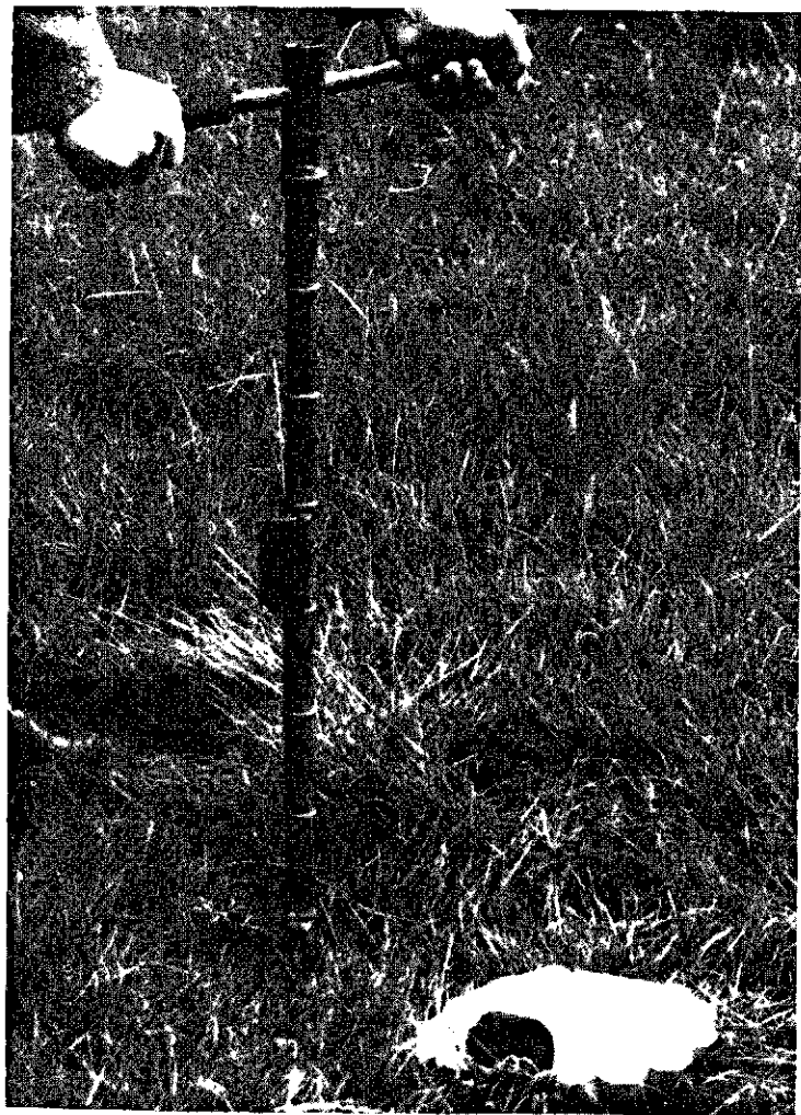
FIG. 13. Drilling a soil sample with a heavy auger
