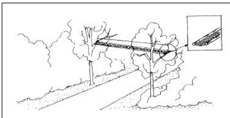
Figure 14. A rope-bridge crossing a road to facilitate a safe passage for red squirrels (Source: Bekker 2002)
