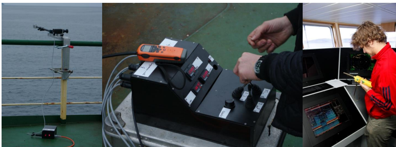
Figure 4 : material developed for the calibration. Left : Metal rod with stepper motor installed on deck; Centre : Steering box on deck, Right : remote steering of the sphere from the bridge
