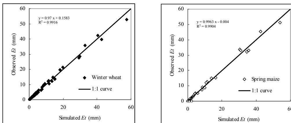
Figure 19. Comparison of simulated and observed value for the contribution from the groundwater to evapotranspiration for winter wheat (1993-1994) and spring maize (1993) in the Central Experimental Station, North China.
