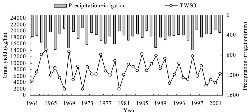
Figure 39. Growing season precipitation + irrigation and simulated grain yield (TWSO) for the period 1961 to 2002 for spring maize under irrigated conditions (single application of 90 mm after jointing) in Taiyuan, Shanxi Province, North China.
