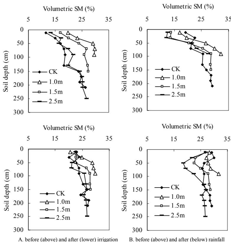
Figure 12. Volumetric soil moisture content variations before and after rainfall and irrigation in the water table depth experiment in the Central Experimental.
