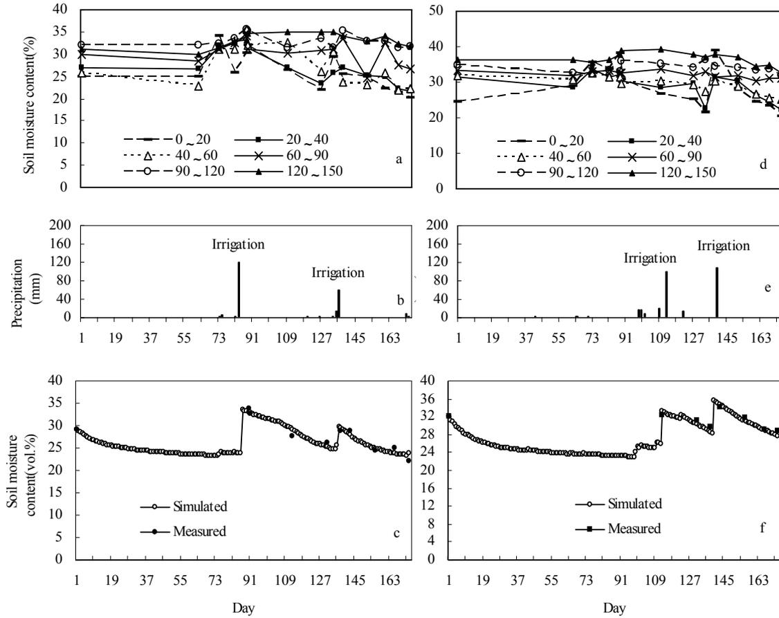
Figure 25. Measured and WOFOST simulated soil moisture content (actual rooting zone) for winter wheat in 1992 (a, b and c) and 1994 (e, f and g) in Central Experimental Station, Shanxi Province, North China.
