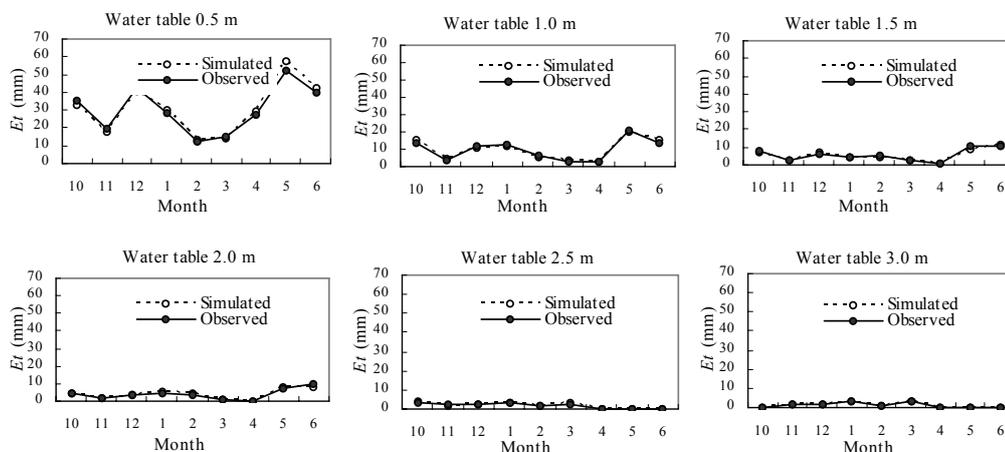
Figure 17. Simulated and observed values for the contribution from the groundwater to evapotranspiration for winter wheat in the 1993-1994 growing season under different groundwater table depths in the Central Experimental Station, North China.
