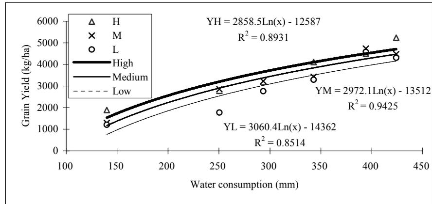
Figure 9. The relation between water consumption and grain yield under high (H, triangles), medium (M, crosses) and low nutrient supply (L, circles) for winter wheat in CES, North China (2004).
