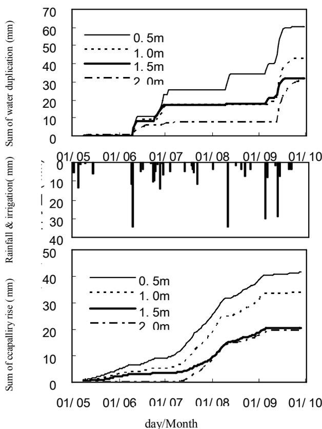
Figure 14. Cumulative drainage (top) and cumulative capillary rise (bottom) and rainfall/irrigation (middle) for the groundwater table experiment depth experiment Transformation of groundwater-soil water under different water table in the Central Experimental Station, North China.
