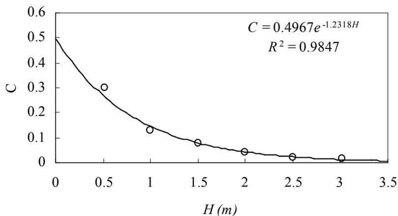
Figure 16. Fitted curve for the relation of the contribution from the groundwater table to evapotranspiration,  $C$  and water table depth  $H$  for a bare soil in the Central Experimental Station, North China (1992).
