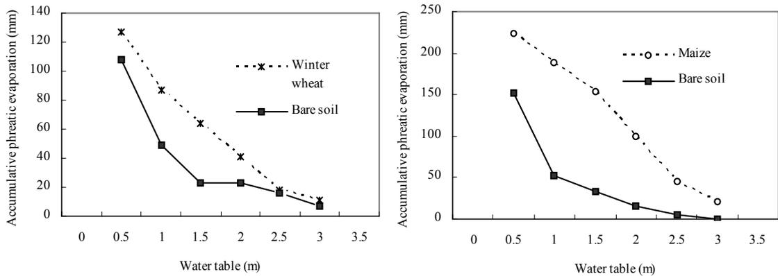
Figure 15. Contribution from the groundwater to evapotranspiration at different water table depths in winter wheat (Oct. 1991 till March 1992) and spring maize (July till September 1992) in the Central Experimental Station, North China.
