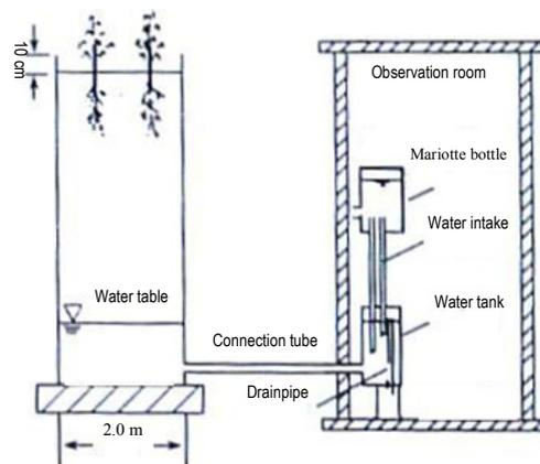
Figure 7. Schematic representation of the groundwater table control facility in the Central Experimental Station, Shanxi Province, North China.
