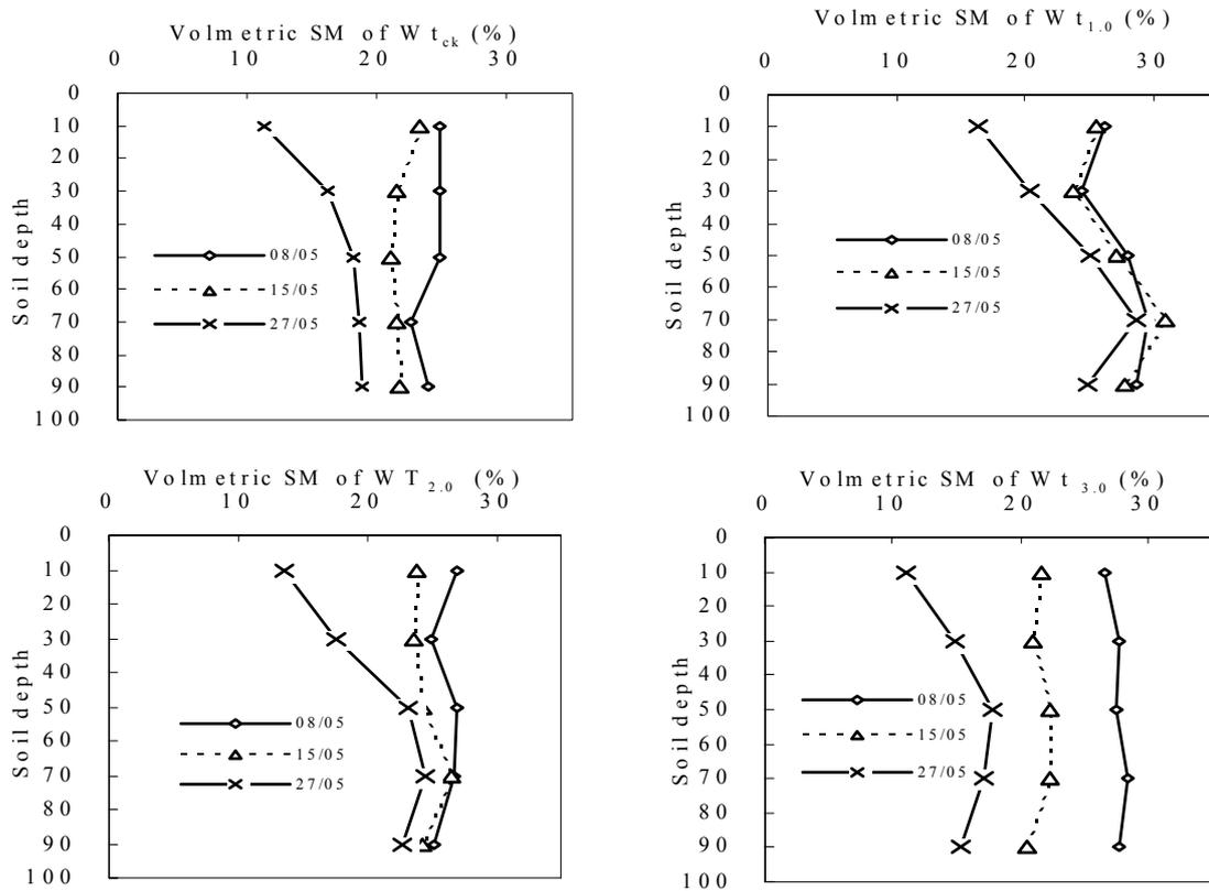
Figure 13. Volumetric soil moisture contents under different water table depths (WT, depth in m.; ck = control) in the water table management experiment in the the Central Experimental Station in North China.
