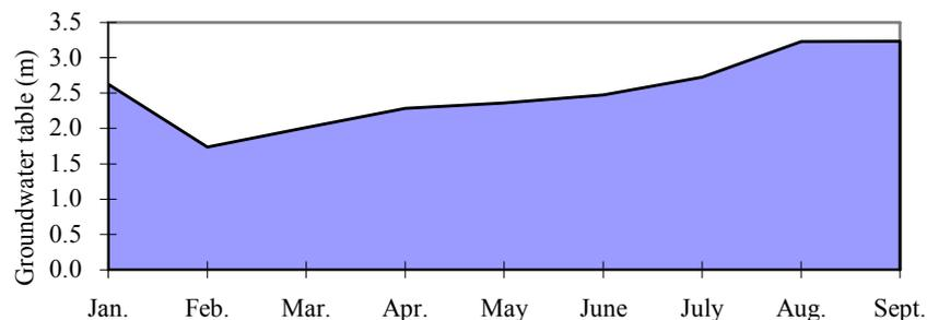
Figure 5. Annual fluctuation in shallow groundwater table depth in the Central Experimental Station, Shanxi Province, North China
