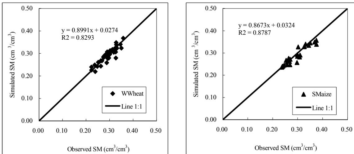
Figure 26. Measured and WOFOST-simulated soil moisture content (potential rooting zone) for winter wheat (1992, 1994, 2001, 2002) (left), and spring maize (2001, 2002) (right) in Central Experimental Station, Shanxi province, North China.
