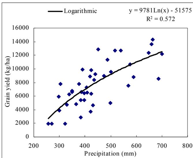
Figure 38. The relation between simulated spring maize grain yield and precipitation+irrigation for the period 1961-2002 in Taiyuan, Shanxi Province, North China.
