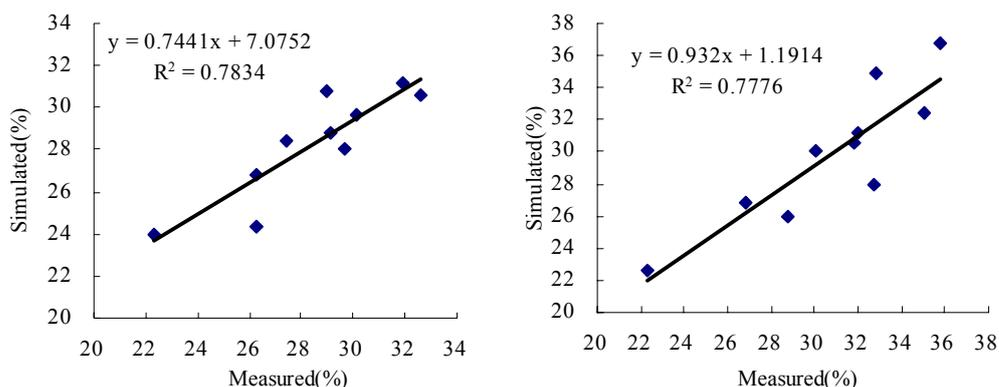
Figure 24. Measured and simulated soil moisture content (actual rooting depth) for winter wheat in 2002 irrigated with 100 mm (left) and 140 mm (right) in two doses in the Central Experimental Station, Shanxi Province, North China.
