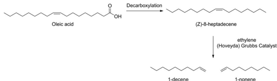
Figure 1. Two step process for the production of Linear Alpha Olefins from oleic acid.
