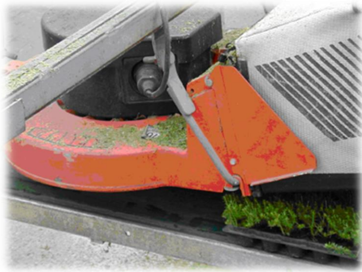
Figure 15 Pruning of Erica by means of a mower on a conveyor belt
