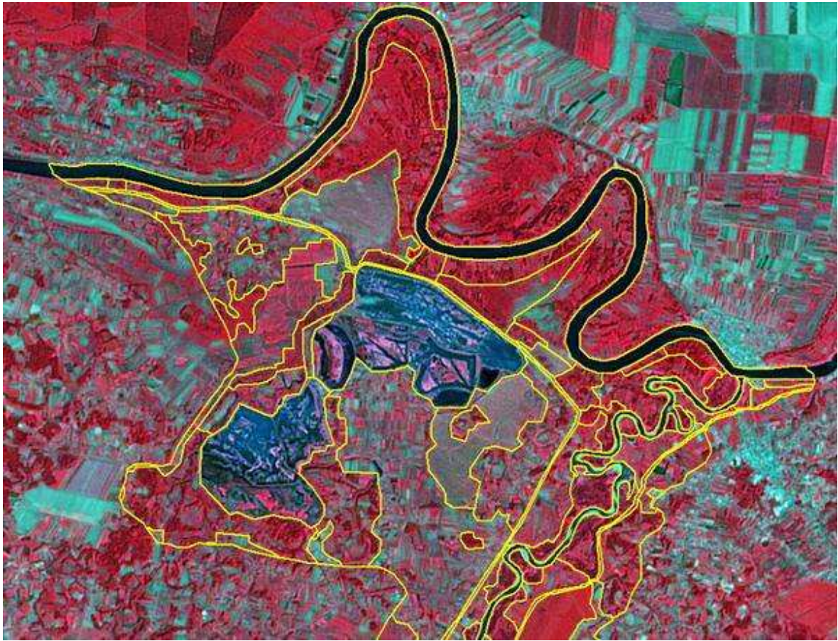
Figure 1 . Pre- delineation of and use categories(polygons )in Baradaca before field work (based on Landsat images)
