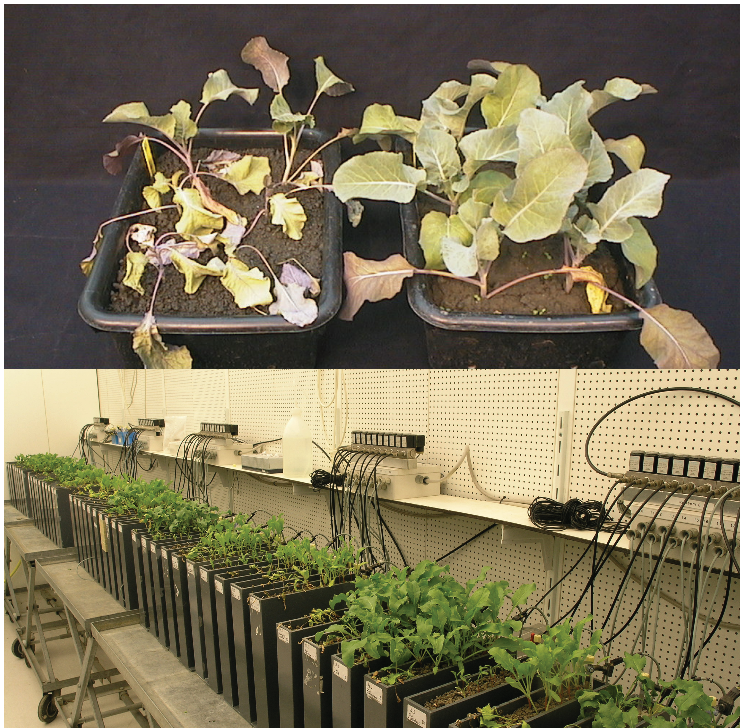
Rhizoctonia symptoms (upper left) and healthy plants with a similar dosage of Rhizoctonia inoculum in a suppressive soil (upper right). Bioassay to assess disease suppression under controlled climate and soil moisture condition (bottom).
