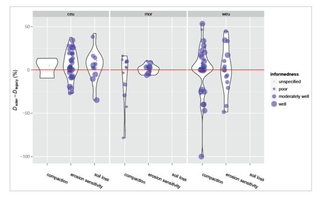
Figure 5-35 Difference between *D*soter and *D*legacy for each NUTS3-unit (blue dots). The size of each dot represents the informedness of the experts.
