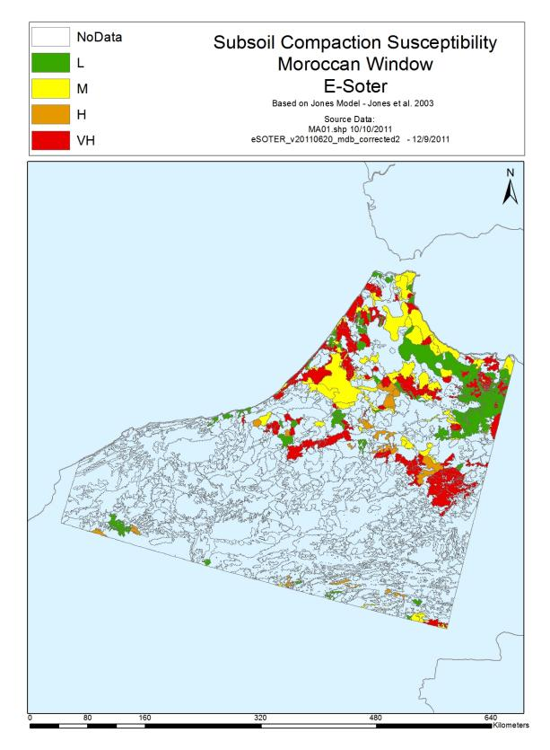
Figure 6. Ma window - Subsoil compaction susceptibility based on E-Soter Database
