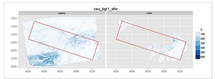
Figure 5-1 Potential soil loss simulated with the BGR model for potential soil erosion (BGR1) using the legacy database (left) and the e-SOTER database (right).
