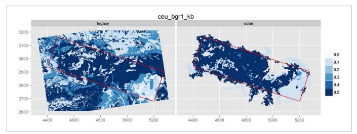
Figure 5-4 Values of the soil factor K<sub>B</sub> based on the legacy database (left) and the e-SOTER database (right).
