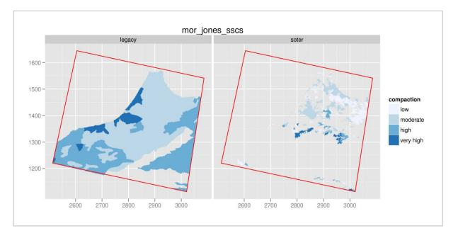
Figure 5-19 Inherent susceptibility to subsoil compaction simulated with the Jones model for the Moroccan window (mor) using the legacy database (left) and the e-SOTER database (right).
