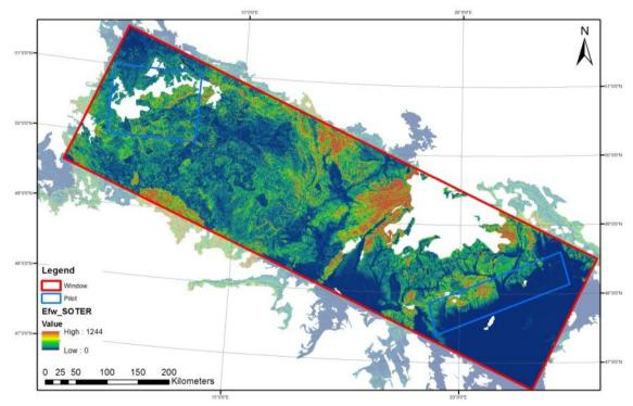
Figure 7: Soil loss by water in t ha<sup>-1</sup> a<sup>-1</sup> using the e-SOTER map as baseline information.
