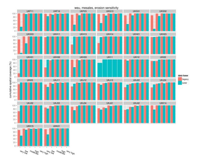
Figure 5-17 Cumulative spatial distributions of erosion sensitivity classes in selected NUTS3 units (in % coverage of the unit) in the West-European window, simulated with the MESALES model using the legacy database (red bars) and the e-SOTER database (blue bars).
