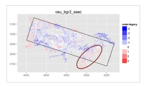
Figure 5-7 Difference in soil sensitivity to water erosion simulated with the BGR2) using the legacy database and the e-SOTER database (difference calculated as output for e-SOTER minus output for legacy database in terms of numbers of classes). Red ellipse indicates area referred to in the text.
