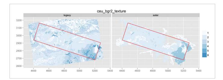
Figure 5-8 Soil texture classes in the CEU window in the legacy database (left) and the e-SOTER database (right). 1: Coarse (<18% clay and > 65% sand), 2: Medium (18% < clay < 35% and >= 15% sand, or <18% clay and 15% < sand < 65%), 3: Medium fine (< 35% clay and < 15% sand), 4: Fine (35% < clay < 60%), 5: Very fine (clay > 60%), 9 (legacy; 0 in e-SOTER): No mineral texture (Peat soils).
