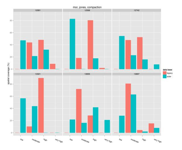
Figure 5-23 Spatial distributions of susceptibility to subsoil compaction classes in selected administrative units (in % coverage of the unit) in the Moroccan window, simulated with the Jones model using the legacy database (red bars) and the e-SOTER database (blue bars).
