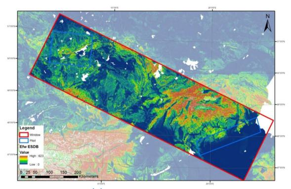
Figure 8: Soil loss by water in t ha<sup>-1</sup> a<sup>-1</sup> using the ESDB map as baseline information.
