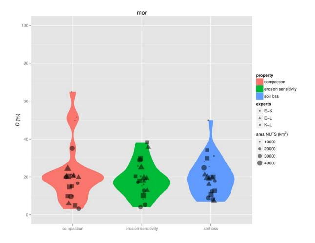
Figure 5-29 'Violin plot' of maximum cumulative difference in spatial distributions of target variables (*D*) assessed by experts for the Moroccan window. Colours distinguish target variables, symbol types distinguish experts, and each individual symbol representing a NUTS3 unit. The size of the symbol indicates the area of the NUTS3 unit in km<sup>2</sup>. The areas of the shapes express the frequency of occurrence of *D*, and represent a unit surface for each target variable.
