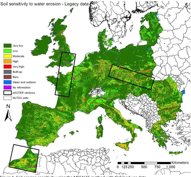
Figure 1. Soil erosion sensitivity using the MESALES method with GLC land use data
