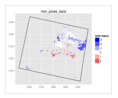
Figure 5-20 Difference in susceptibility to subsoil compaction simulated with the Jones model between the legacy database and the e-SOTER database (difference calculated as output for e-SOTER minus output for legacy database in terms of numbers of classes).
