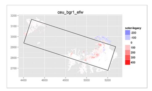
Figure 5-2 Difference in potential soil loss simulated with the BGR model for potential soil erosion (BGR1) using the legacy database and the e-SOTER database (difference calculated as output for e-SOTER minus output for legacy database).
