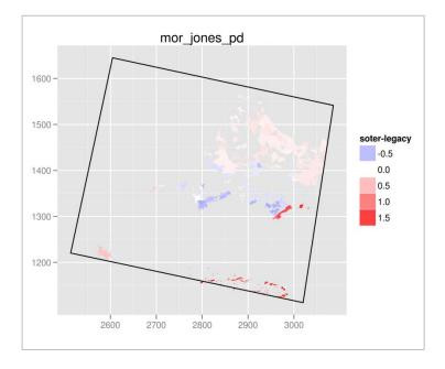
Figure 5-22 Difference in packing density in the Jones model application between the e-SOTER and legacy databases for the West-European window (in t\*m<sup>-3</sup>). Difference calculated as model variable in application using the e-SOTER database minus the model variable in the legacy database.
