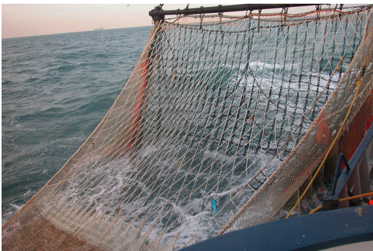
Figure 23. Large mesh (1.20m) top panel in a chain-mat round net
