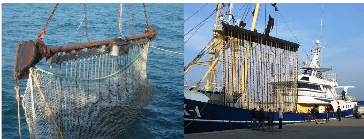
Figure 32. Flatfish pulse beam trawls, left DELMECO 2005; right HFK 2011.
