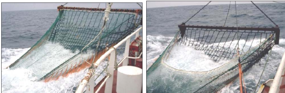
Figure 28 Square mesh top panels (left) and Cutaway covers (right)
