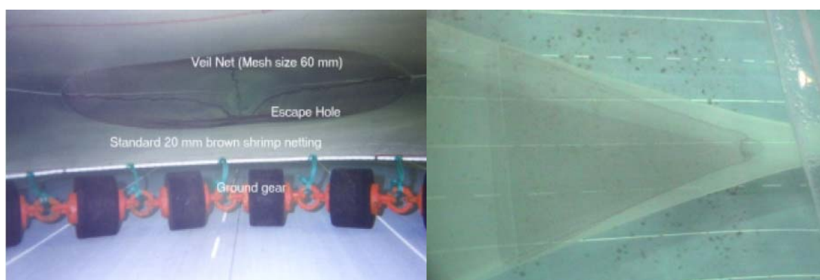
Figure 33. Sieve or veil net developed for the Crangon fishery.
