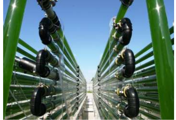
Vertical stacked tubular reactor
