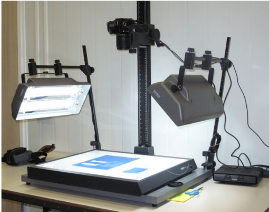
Figure 1. The image acquisition setup, consisting of a standard repro stand, a digital single-lens reflex (DSLR) camera (Nikon D90) with 50mm lens and adjustable high frequency front and back light.
