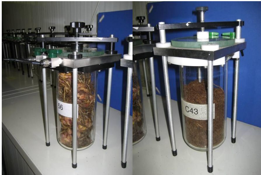
Figure 18: closed bottles for \text{CO}_2 -production measurements; left bulbs; right peat.
