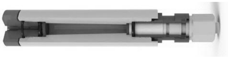
Figure 6.2. Schematic representation of the micro-RFC column from Proxcys (Nieuw-Amsterdam, The Netherlands). Inward flow is mimicked by liquid flow from left to right, outward flow vice versa. This picture was reproduced with permission from Proxcys.
