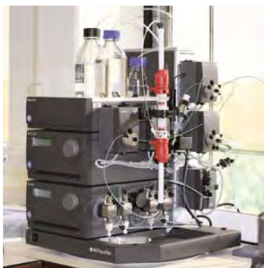
Figure 1.1. Example of a lab scale preparative chromatography setup with an Äkta Purifier (GE Healthcare, Uppsala, Sweden).
