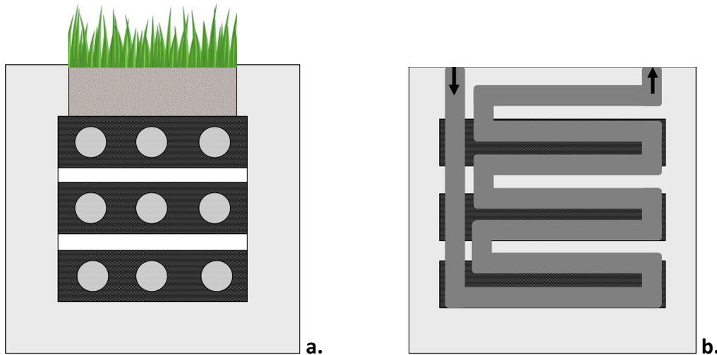
*Figure 4.3: Anode (3a) and cathode (3b) schematic overview of a flat-plate Plant Microbial Fuel Cell. In anode and cathode top, middle and bottom sections are shown; in anode sample-points are shown; and in cathode the flow-through channel is shown.*
