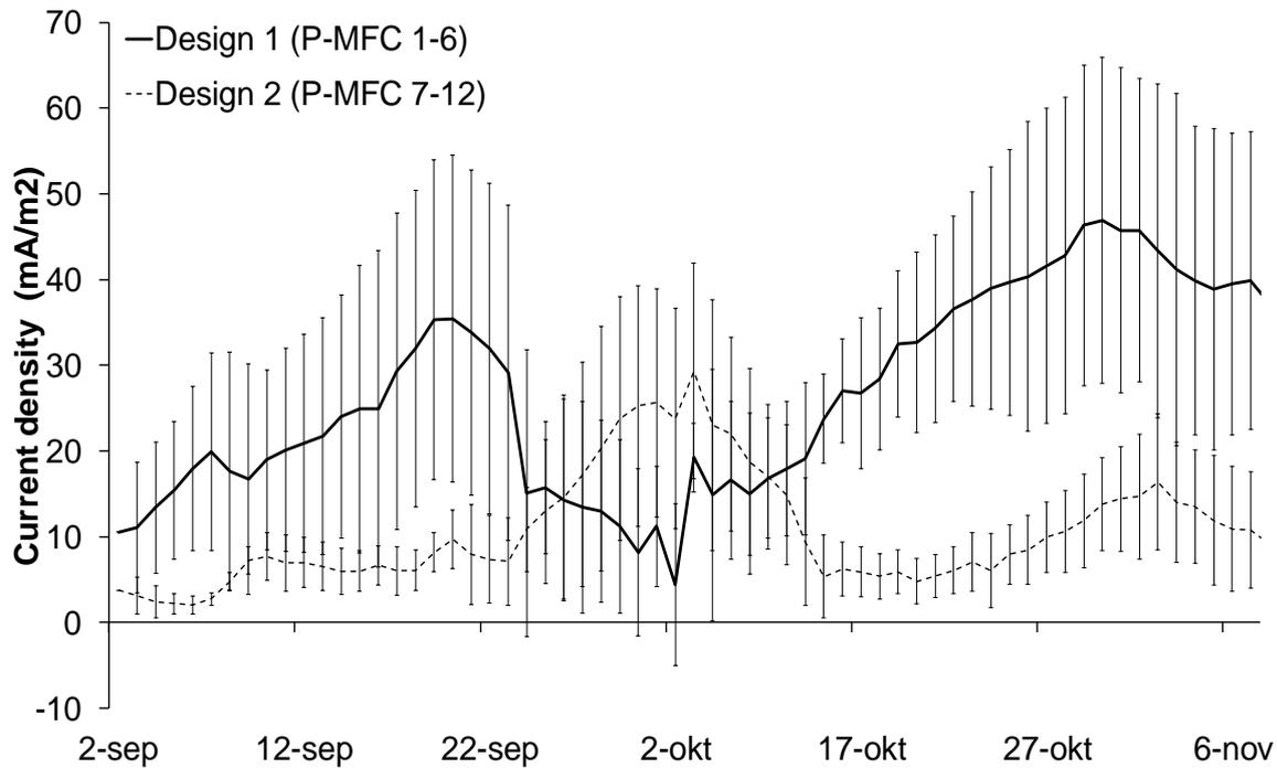
*Figure 5.2: Average current density of two designs of Plant-Microbial Fuel Cells (6 per design) during first two months of experimental runtime, in which design 1 has a shorter start-up time than design 2, but both designs start-up within the first two months. Error bars represent standard deviation of average.*
