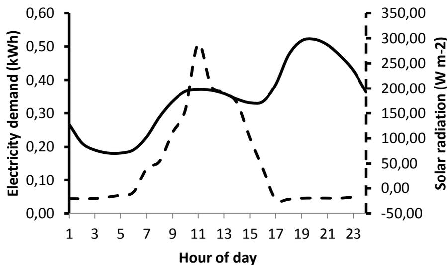
*Figure 1.4: Electricity demand (kWh) of a Dutch household during the day in autumn (41) compared to average solar radiation during a day in September 2009 (W m<sup>-2</sup>)(42).*
