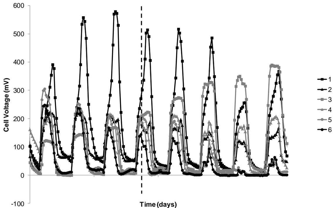
*Figure 5.8: P-MFC 1-6 (design 1) before and after changing external resistance of P-MFC 1, 2, 6 to 500  $\Omega$  from 900  $\Omega$  and leaving P-MFC 3, 4, 5 at 900  $\Omega$  external resistance. Dashed line is moment of changing external resistance of P-MFC 1, 2 and 6. After changing external resistance no direct effect can be observed. After 3 days cell potential of P-MFC 6 drops.*
