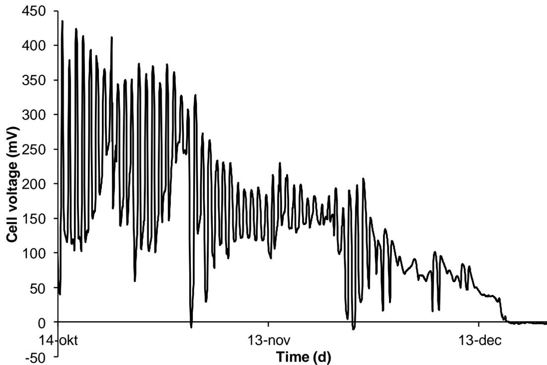
Figure 5.3: Diurnal cycle in cell voltage of P-MFC 1 as an example of diurnal cycles that were observed from start-up almost until first frost period on December 23. P-MFC 2 and P-MFCs 7-12 showed a similar pattern (data not shown).
