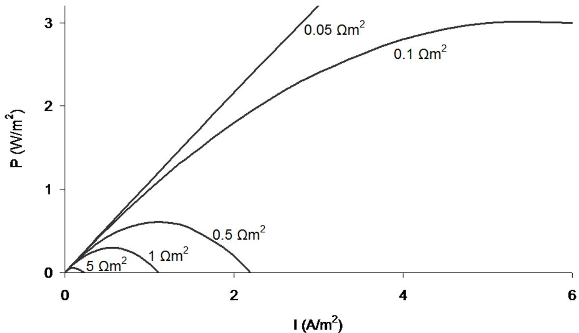
Figure 7.3: Power density as function of current density at different internal resistances, based on  $P = P_{max} - I^2 R_{int}$
