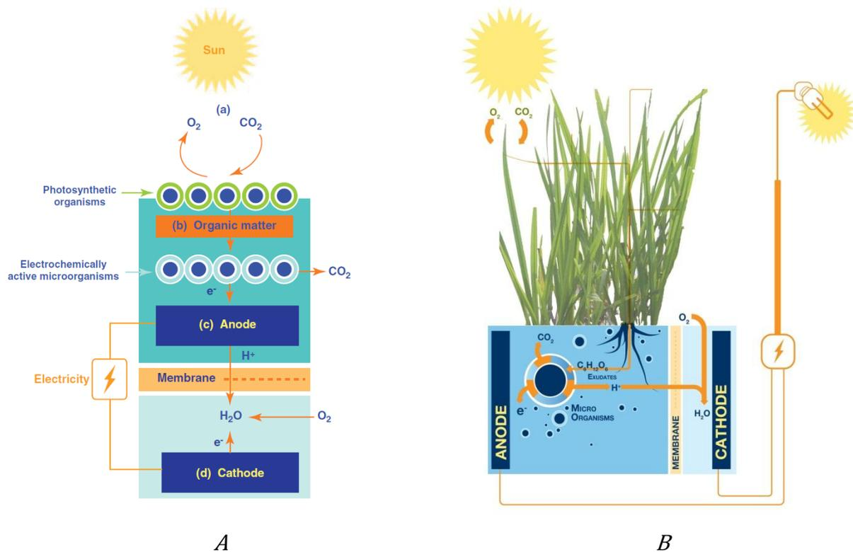
*Figure 1.3: Schematic overview of a Microbial Solar Cell (MSC) (A) of which the Plant-Microbial Fuel Cell (P-MFC) (B) is a specific type. In the P-MFC the photosynthetic organisms are plants.*
