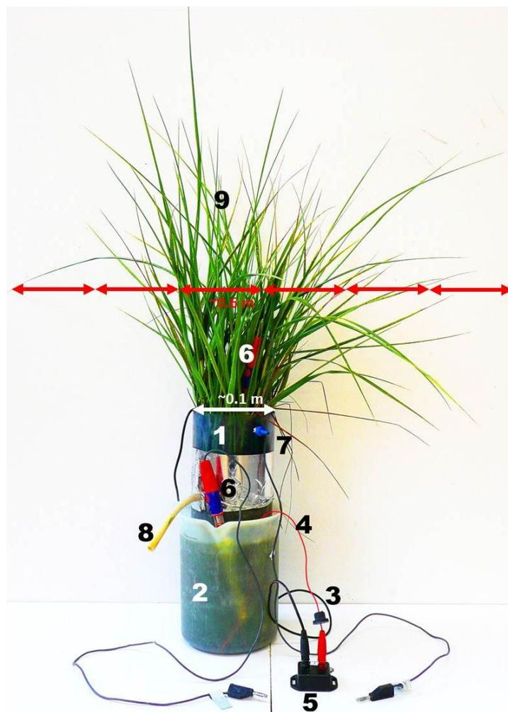
*Figure 7.1: Experimental set-up from chapter 2, in which maximum width of above ground biomass is approximately 6 times width of anode.*
