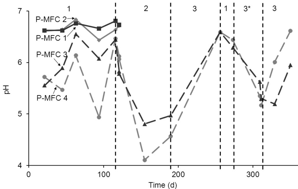
*Figure 3.4 pH measurements during the 365 days of experiment with different plant-growth media. Changes in plant-growth medium are indicated with dotted lines. 1 = modified Hoagland medium 50%, 2 = nitrate-less, ammonium-chloride-rich medium, 3 = nitrate-less, ammonium-bicarbonate-rich medium*
