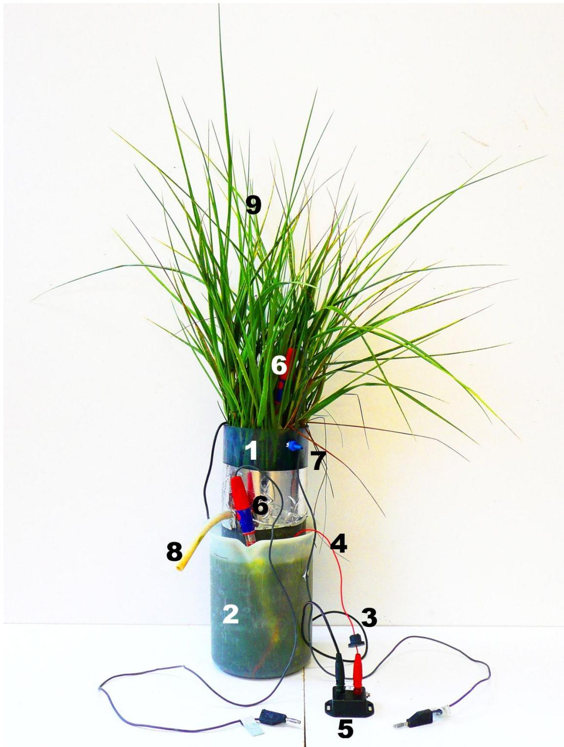
*Figure 2.4: Experimental set-up, in which 1= anode compartment, 2=cathode compartment, 3=anode wire, 4= cathode wire, 5=external resistance, 6=reference electrode, 7=water and plant-growth medium filling point, 8=anode overflow, 9=Spartina anglica*
