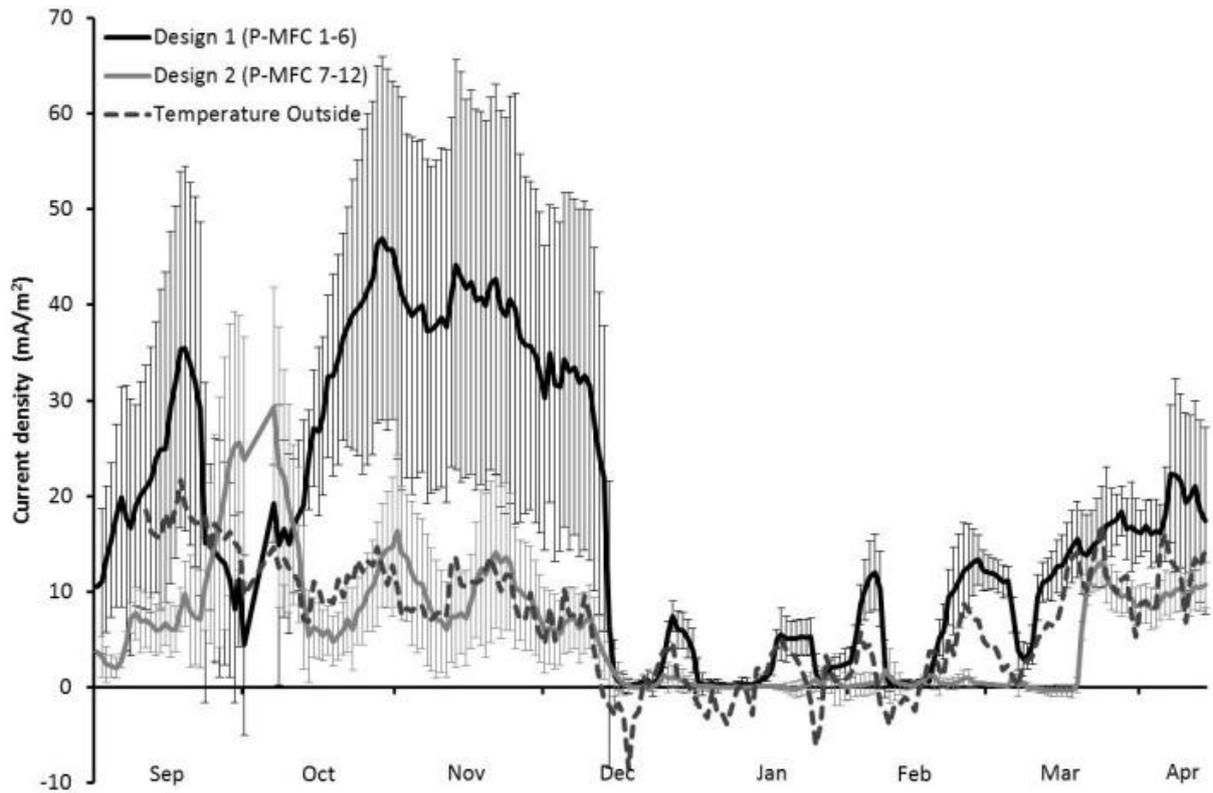
Figure 5.6: Average current densities (mA/m<sup>2</sup>), including standard deviation, of P-MFCs of design 1 (P-MFC 1-6) and design 2 (P-MFC 7-12) during complete runtime of the experiment in which design 1 shows consistently higher current densities than design 2.
