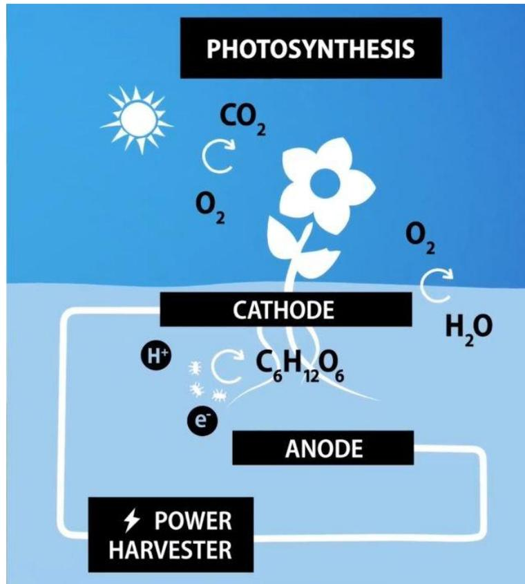
*Figure 6.1: Schematic overview of Plant-Microbial Fuel Cell (13)*
