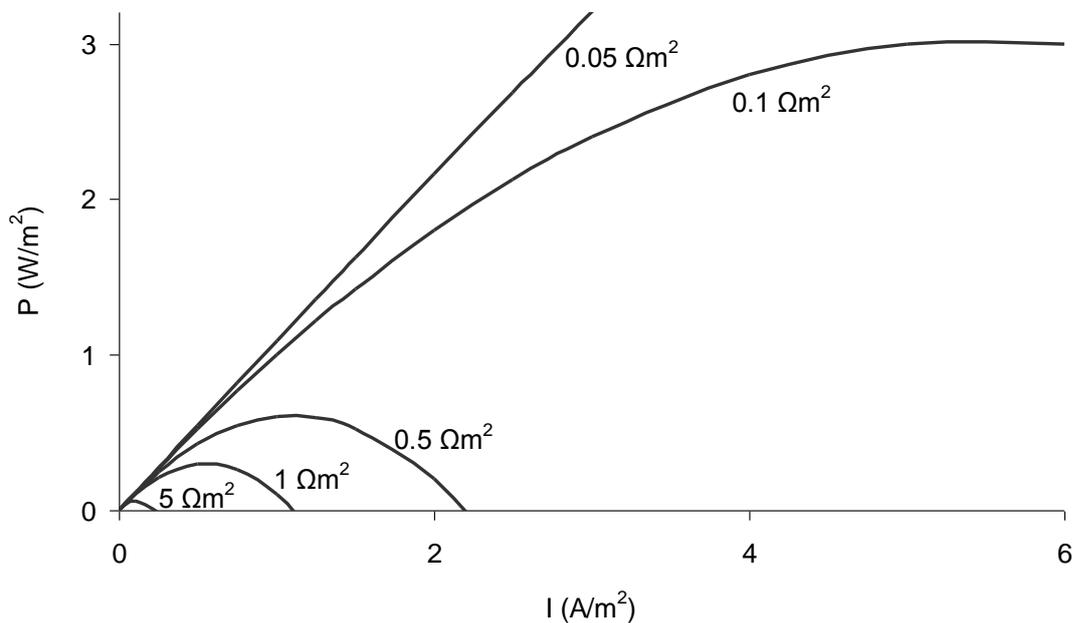
*Figure 4.1: Power density as a function of current density at different internal resistances, which shows that internal resistance should be  $<0.094 \Omega \text{ m}^2$  to achieve a power density of  $3.2 \text{ W/m}^2$*
