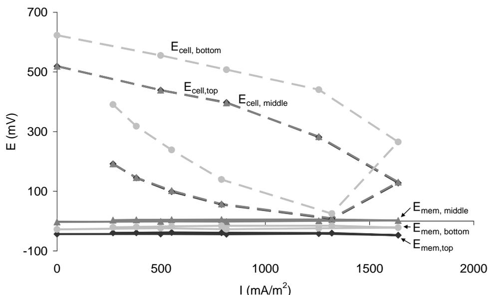
*Figure 4.6: Membrane voltages ( $E_{mem}$ ) and cell voltages ( $E_{cell}$ ) as a function of current density in top, middle and bottom sections of P-MFC 2 during polarization curve on day 320, in which membrane voltages stay low with increasing current, indicating a small membrane resistance.*
