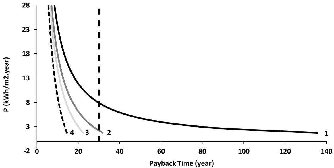
*Figure 7.4 Payback time – when energy input in system equals energy output – of the P-MFC based on different power output of the P-MFC ranging from  $1.75 \text{ kWh m}^{-2} \text{ year}^{-1}$  to  $28 \text{ kWh m}^{-2} \text{ year}^{-1}$  ( $0.2 \text{ W m}^{-2}$  –  $3.2 \text{ W m}^{-2}$ ) for four scenarios: 1) without co-products, 2) with heat insulation as a co-product, 3) with biogas production as a co-product, and 4) with both heat insulation and biogas production as co-products.*
