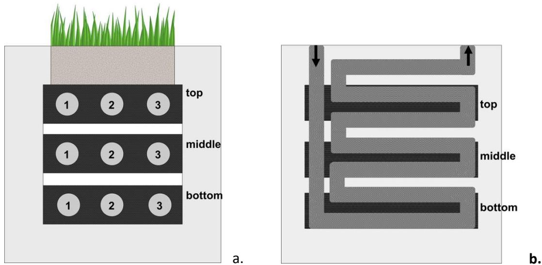
*Figure 3.2: Anode (a) and cathode (b) schematic overview of a flat-plate Plant-Microbial Fuel Cell. In anode and cathode top, middle and bottom sections are indicated; in anode sample-points are indicated with numbers 1, 2 and 3; and in cathode the flow-through channel is shown. Anode and cathode were assembled with top, middle and bottom sections of anode and cathode against each other, separated by a membrane.*
