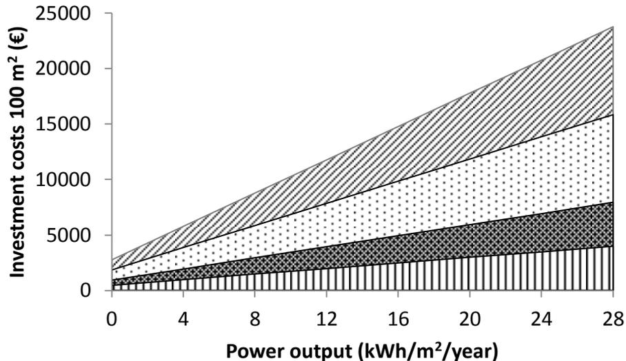
*Figure 7.6: Investment costs for 100 m<sup>2</sup> of Green Electricity Roof at increasing power output. For a pay-back time of maximum 30, 20, 10 and 5 years investment costs should be in the shaded area of the graph. Highest line is 30 years, lowest 5 years.*
