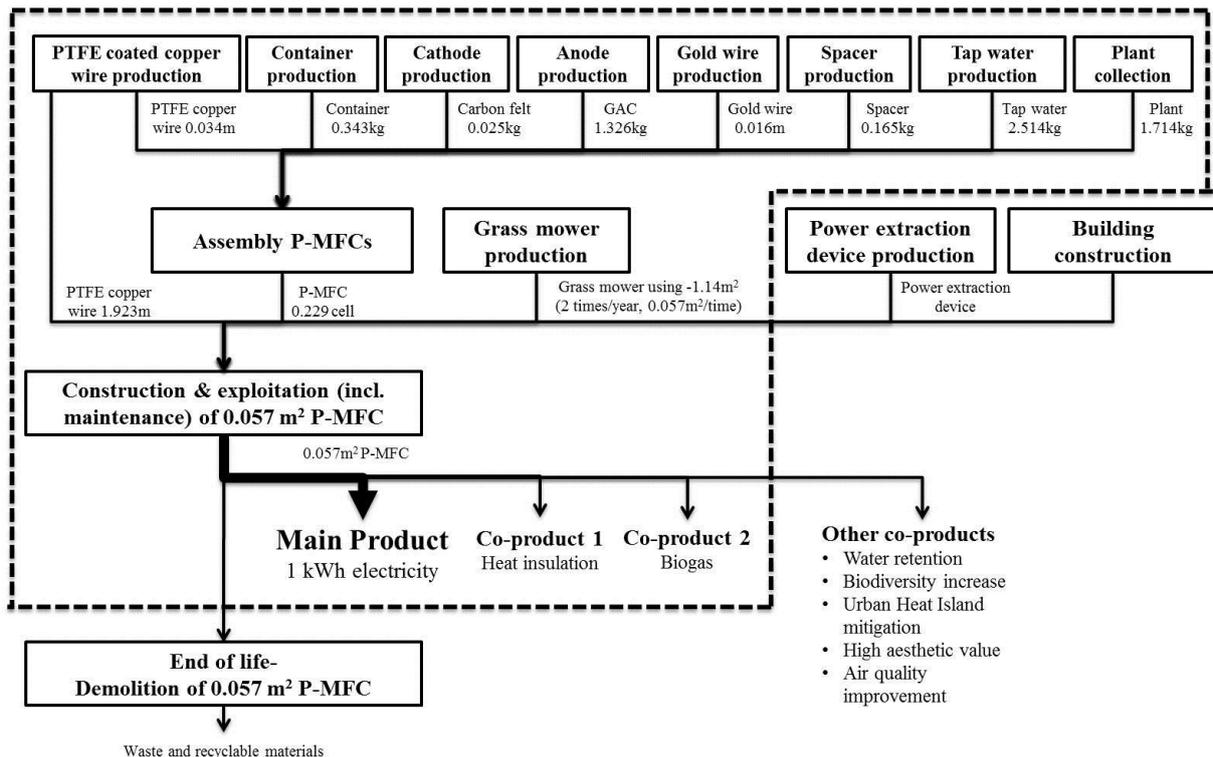
Figure 6.2: Flow chart of a P-MFC to produce and supply 1 kWh electricity to the grid of the building on the pilot on the NIOO-roof. The quantified flows relate to the reference scenario in this LCA with 1.75 kWh/m<sup>2</sup>/year electricity production. The dotted line generically indicates the system boundaries for all scenarios; inclusion of heat insulation and biogas differ between scenarios.
