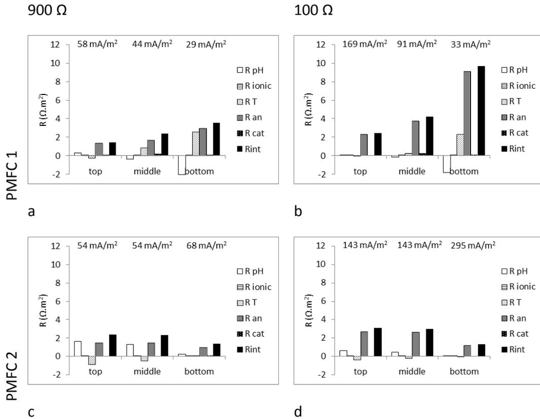
Figure 4.5: Partial and total internal resistances ( $\Omega.m^2$  membrane surface area) at three different depths (top, middle, bottom) in two P-MFCs on day 320 of experiment at 900  $\Omega$  and 100  $\Omega$  external resistance.
