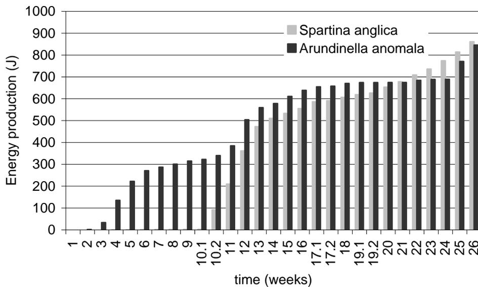
Figure 2.2: Electricity production of *Spartina anglica* and *Arundinella anomala* in a P-MFC during 26 weeks of experiment. Some weeks are split in two parts, indicated with .1 and .2, because of changing conditions. 10.2 = change of catholyte *Arundinella anomala* from buffer to ferric cyanide. 17.2 = change of external resistance at start of maximization strategy. 19.2 = change of external resistance at end of maximization strategy.
