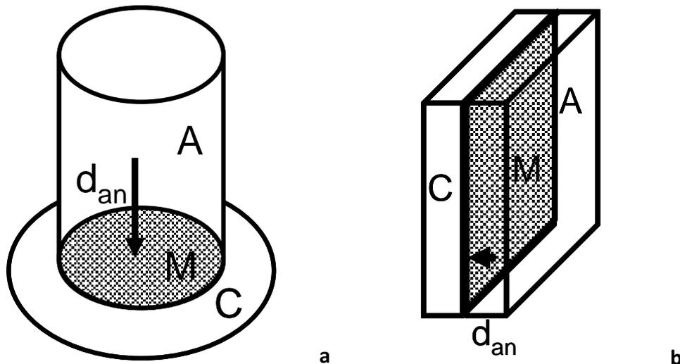
Figure 4.2: Tubular (2a) and flat-plate (2b) design of a Plant Microbial Fuel Cell, in which A=anode, C=cathode, M=membrane,  $d_{an}$ = average distance between anode and membrane. Distance between anode and membrane is shorter in flat-plate design than in tubular design.
