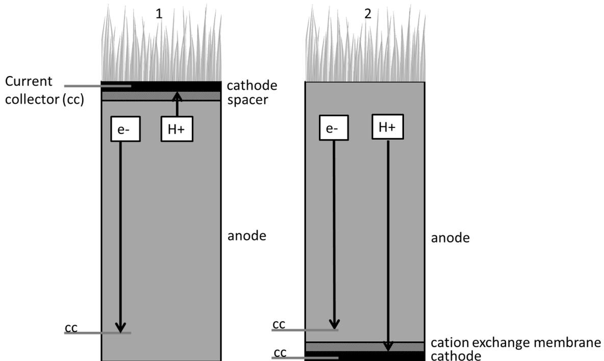
Figure 5.1: Schematic representation of Plant-Microbial Fuel Cells of design 1 (left) and design 2 (right) that were placed on a roof-top in Wageningen, the Netherlands.
