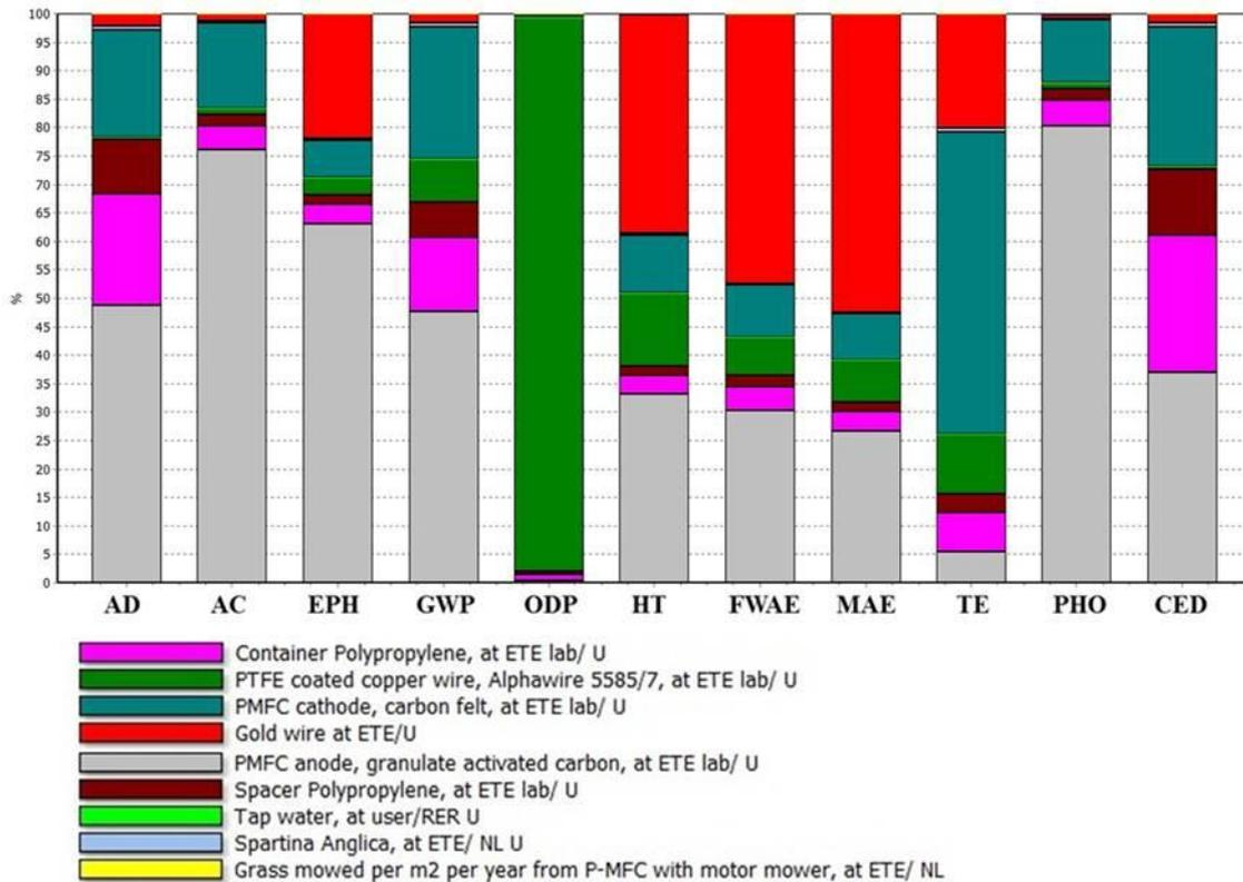
Figure 6.4: The contributions of the different parts of the P-MFC construction and grass mowing to the selected impact categories (calculated for 1 kWh electricity supply in the reference scenario), in which AD=Abiotic Depletion, AC=Acidification, EPH=Eutrophication, GWP=Global Warming Potential, ODP=Ozone Depletion, HT=Human Toxicity, FWAE=Fresh Water Aquatic Ecotoxicity, MAE=Marine Aquatic Ecotoxicity, TE=Terrestrial Ecotoxicity, PHO=Photochemical Oxidation.
