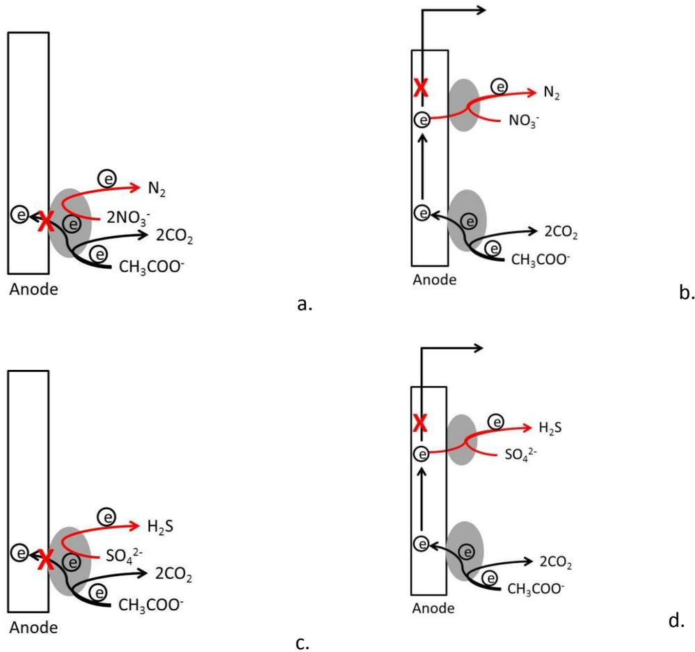
*Figure 3.1: Two pathways of nitrate reduction (a, b) and sulphate reduction (c, d) at the anode of a Plant-Microbial Fuel Cell. In pathway 1 (a, c) electrons released in the oxidation of organic matter are directly used by the same organism for nitrate or sulphate reduction. In pathway 2 (b, d) electrons released in the oxidation of organic matter and donated to the anode are taken from the anode by another organism for nitrate or sulphate reduction.*
