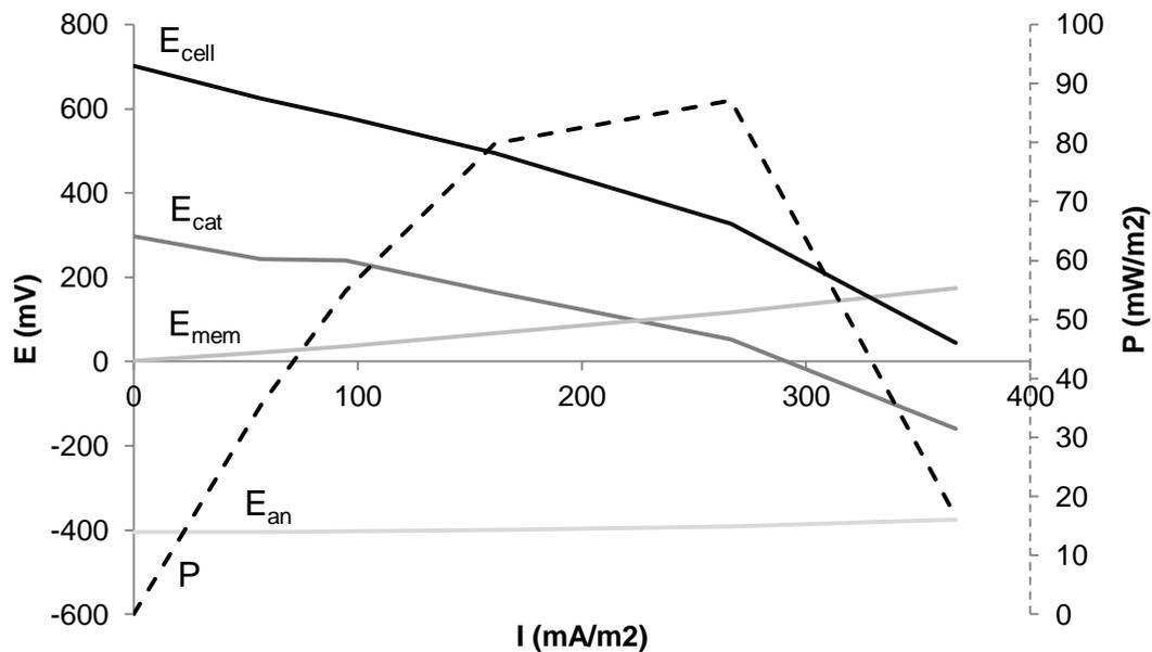
Figure 5.5: Polarisation curve of P-MFC 1 in which cathode is limiting maximum power output.
