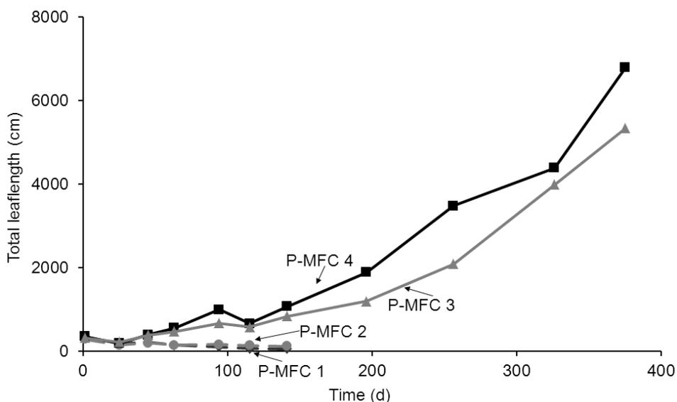
*Figure 3.3: Plant-growth during 365 days of experiment in cm. P-MFC 1 and 2 were fed plant-growth medium with phosphate buffer, P-MFC 3 and 4 were fed plant-growth medium without phosphate buffer. Plant-growth measurement of P-MFC 1 and 2 was stopped after day 145 because of plant-death. Relative plant-growth was variable over the year.*
