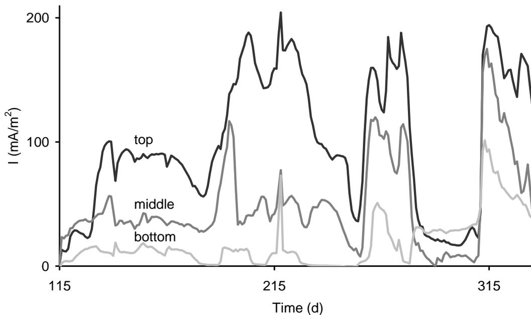
*Figure 4.4: Electricity production ( $\text{mA}/\text{m}^2$ ) in top, middle and bottom sections of P-MFC 1 during day 115 through 337 in which top section produces most electricity. Fluctuations in power output over time are caused by changes in medium composition as described in Helder et al. 2011 [13].*
