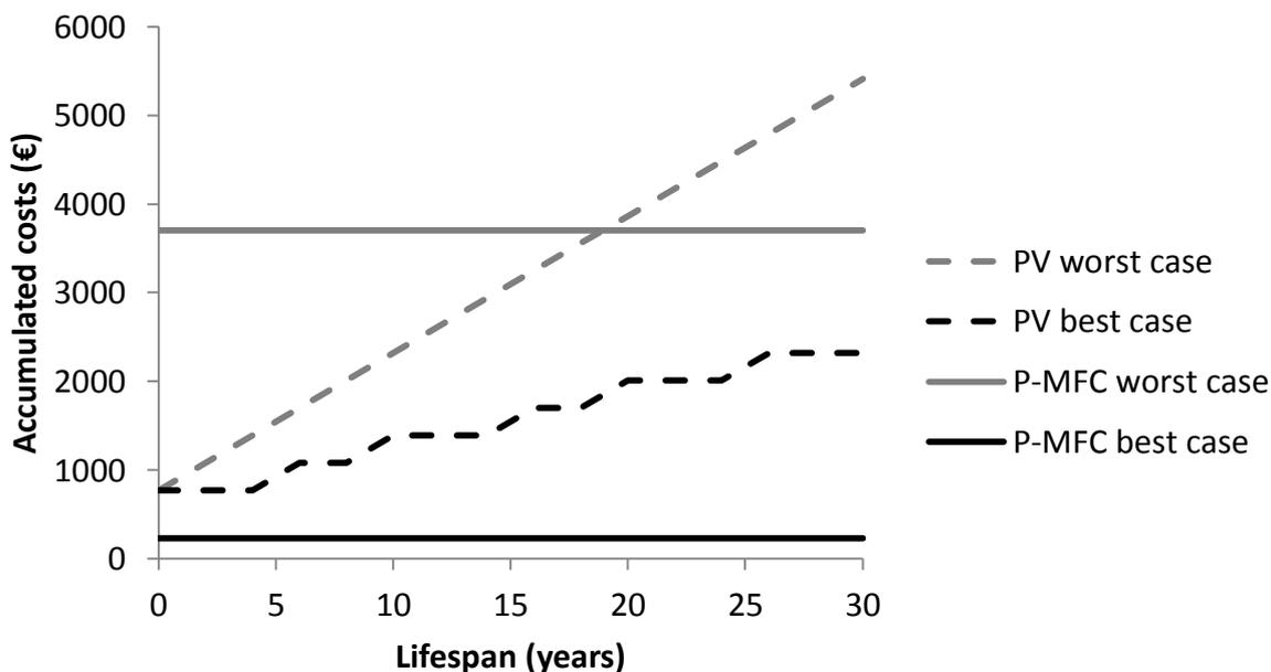
*Figure 7.7: Accumulated costs over a 30 years lifespan of a stand-alone PV solar system and a stand-alone P-MFC system. PV worst case is with a lifespan of the battery pack of 2 years, PV best case is with a lifespan of the battery pack of 5 years. P-MFC worst case is based on  $0.2 \text{ W m}^{-2}$  and optimized costs of  $\text{€}9.26 \text{ m}^{-2}$ , P-MFC best case is  $3.2 \text{ W m}^{-2}$  and optimized costs of  $\text{€}9.26 \text{ m}^{-2}$ .*
