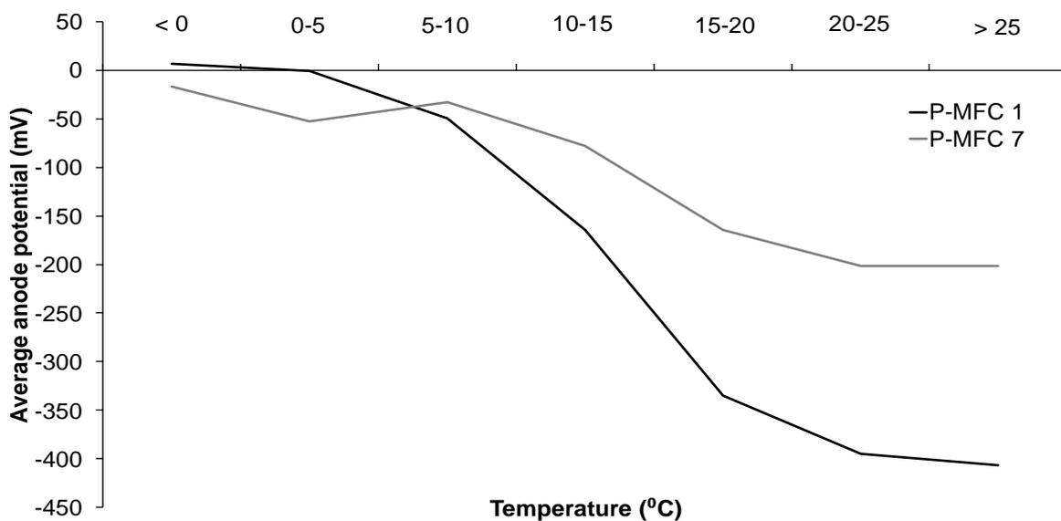
Figure 5.9: Average anode potential of P-MFC 1 and P-MFC 7 over all measurements ( $n=4695$ ) in relation to temperature.
