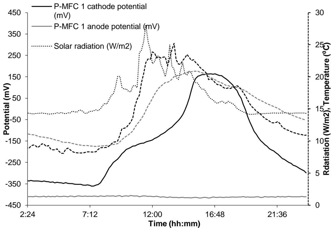
Figure 5.4: Development of anode and cathode potential of P-MFC 1 during 24 hours in relation to solar radiation and temperature, in which cathode potential shows a diurnal cycle.
