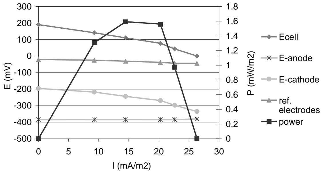
*Figure 2.3: Polarization curve *Arundinella anomala* showing a stable anode potential and decreasing cathode potential, indicating that the reaction at the cathode is the limiting factor in power production.*
