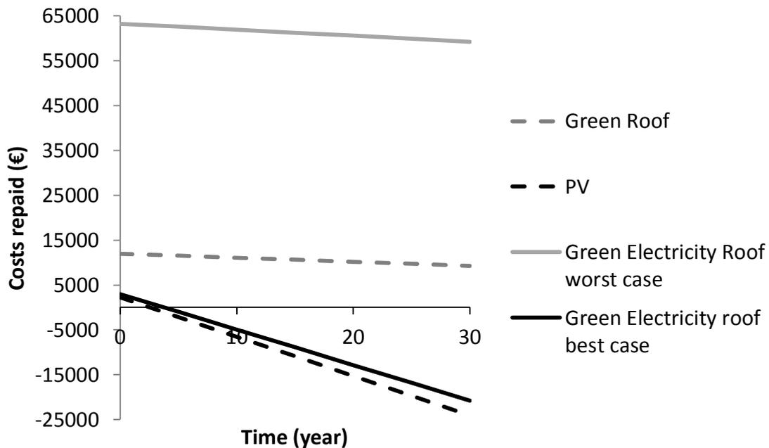
*Figure 7.5 Investment-costs and pay-back time of normal green roofs, PV solar panels and the Green Electricity Roof in three scenario's. Worst case scenario is current state of technology and pricing ( $0.2 \text{ W/m}^2$  and  $\text{€}630./\text{m}^2$ ). Best case is maximum power output and minimum costprice ( $3.2 \text{ W/m}^2$  and  $\text{€}30./\text{m}^2$ ).*
