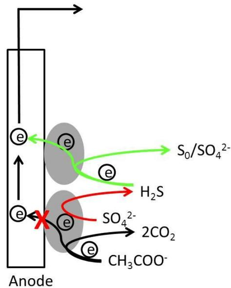
*Figure 3.6: Re-oxidation of hydrogen-sulphide to solid sulphur at the anode of a Plant-Microbial Fuel Cell, regaining electrons for electricity production*
