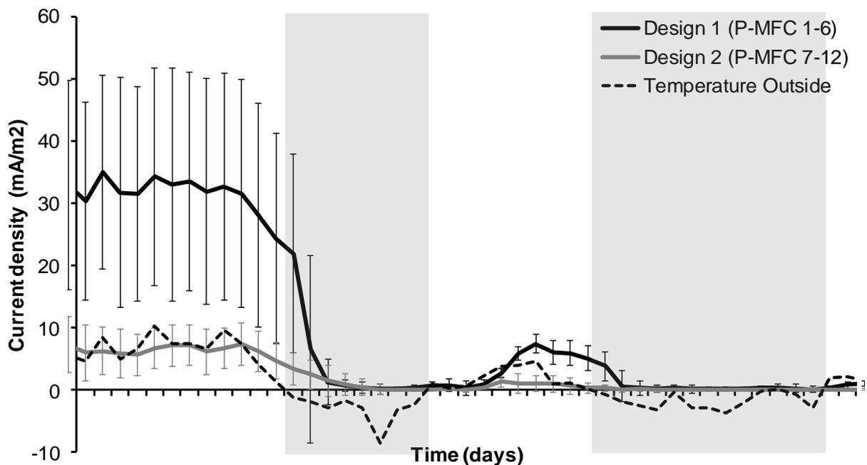
Figure 5.7: Average current densities over 6 P-MFCs of design 1 and 6 P-MFCs of design 2 at low temperatures. Grey areas represent frost periods. Current production continues shortly after frost sets in. Error bars represent standard deviation from average.
