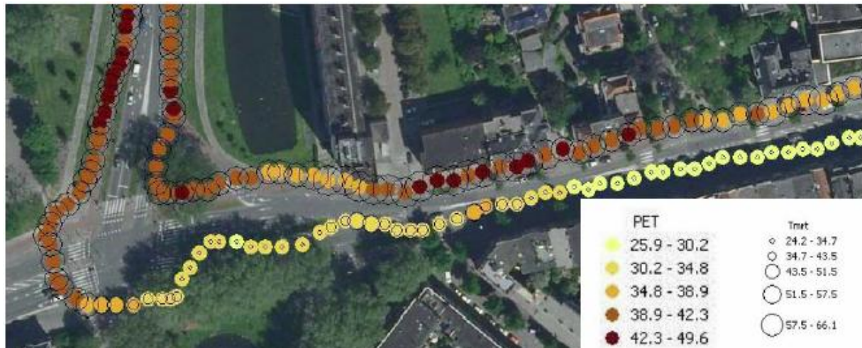
Figure 5.1.: PET (colours) and radiation exposure (circles) afternoon, August 6, 2009
