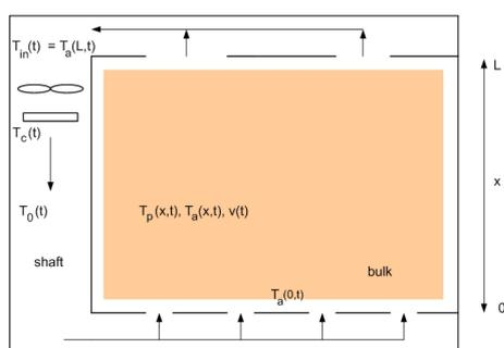
**Figure 1:** Schematic representation of a bulk storage room.
