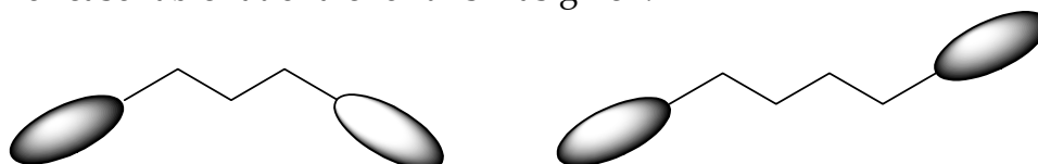
Figure 5. Schematic representation of dimeric molecules with an odd and an even number of flexible units between the two mesogens.
