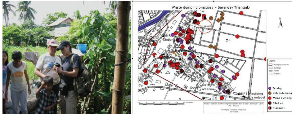
Figure 3.7: GIS-based transects carried out with ward officers (left) and output of GIS-direct mapping for waste dumping practices in Triangulo (right).
