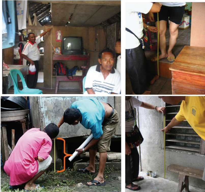
Figure 6.2 Measurement of water depth reached by flood events according to people's remembrances (lower two pictures by Saut Sagala).
