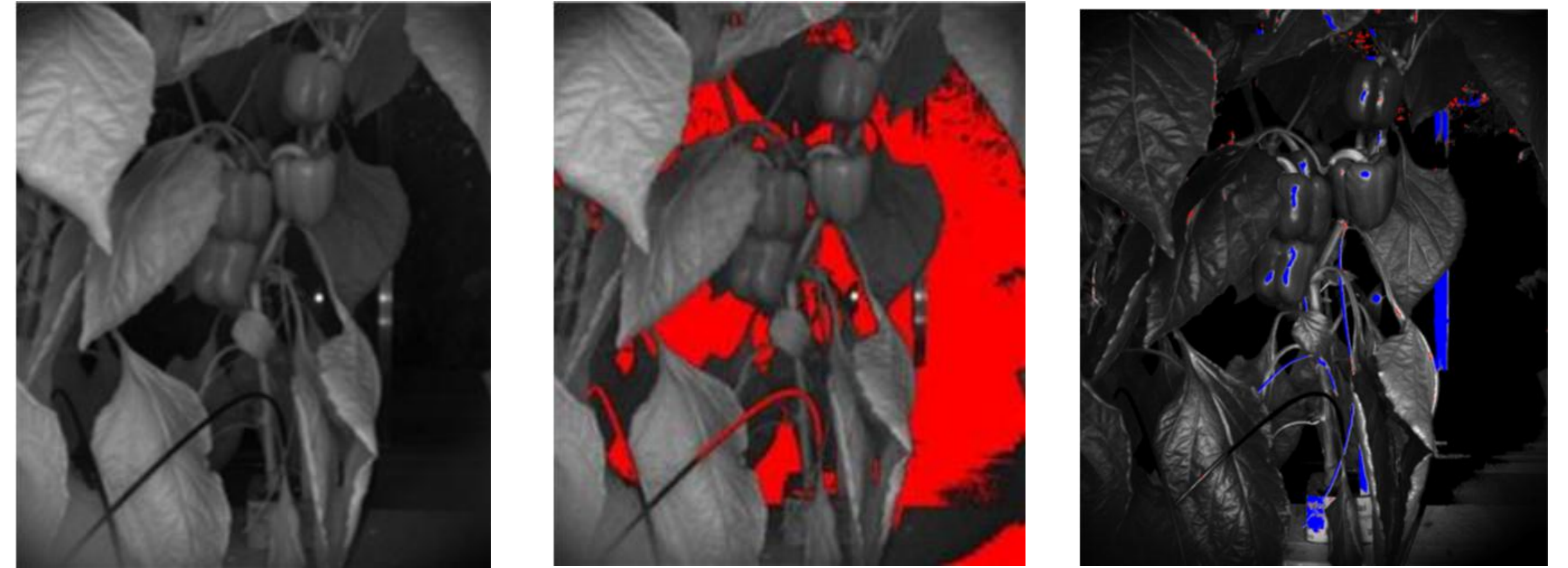
Figure 3. Original image at wavelength >900 nm (left) and threshold operation (middle). Overexposed regions (>300 pixels) are classified as hard obstacles and smaller regions are removed (right)
