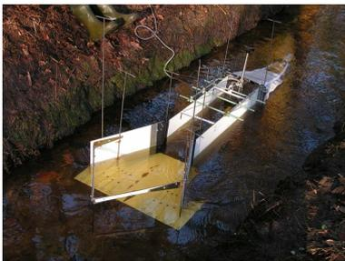
fig 2. Apparatus used to increase the current velocity in the experimental area.
