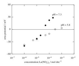
Figure 4. Zeta-potentials measured at pH = 5.8 and 7.3 as a function of the La(NO $_3$ ) $_3$  concentration. pAg = 12.2; c<sub>KNO $_3$ </sub> = 1 mmol dm<sup>-3</sup>.
