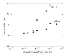
Figure 5. Zeta-potentials measured at pH = 4 and pH = 5 as a function of the Al(NO<sub>3</sub>)<sub>3</sub> concentration. pAg = 12.2;  $c_{KNO_3} = 1 \text{ mmol dm}^{-3}$ .
