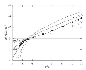
Figure 1. Surface charge of silver iodide as a function of the Ag concentration at different concentrations of KNO $_3$  measured at pH = 5.8. For comparison data taken from Ref. 6 are also shown (solid lines).
