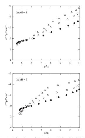
Figure 3. Surface charge of silver iodide in  $10^{-3}$  mol dm<sup>-3</sup> KNO<sub>3</sub> measured at pH = 4 (panel (a)) and pH = 5 (panel (b)) as a function of the Ag concentration in the absence (closed symbols) and in the presence of Al(NO<sub>3</sub>)<sub>3</sub> (open symbols). Al(NO<sub>3</sub>)<sub>3</sub> concentration:  $\bullet$  – 0 mol dm<sup>-3</sup>, o –  $10^{-4}$  mol dm<sup>-3</sup>,  $\Delta$  –  $10^{-3}$  mol dm<sup>-3</sup>.
