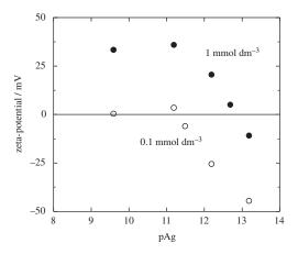
Figure 6. Zeta-potentials measured in 0.1 mmol dm $^{-3}$  and 1 mmol dm $^{-3}$  La(NO<sub>3</sub>)<sub>3</sub> solutions at pH = 7.
