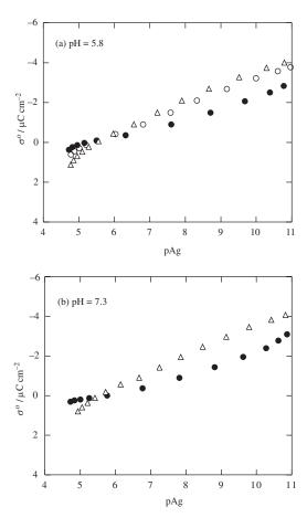
Figure 2. Surface charge of silver iodide in  $10^{-3}$  mol dm<sup>-3</sup> KNO<sub>3</sub> measured at pH = 5.8 (panel (a)) and pH = 7.3 (panel (b)) as a function of the Ag concentration in the absence (closed symbols) and in the presence of La(NO<sub>3</sub>)<sub>3</sub> (open symbols). La(NO<sub>3</sub>)<sub>3</sub> concentration:  $\bullet$  – 0 mol dm<sup>-3</sup>, o –  $10^{-4}$  mol dm<sup>-3</sup>,  $\triangle$  –  $10^{-3}$  mol dm<sup>-3</sup>.
