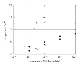
Figure 7. Zeta-potentials measured at pH = 7 (closed symbols) and pH = 9 (open symbols) as a function of the  $Ca(NO_3)_3$  (o) and  $Zn(NO_3)_3$  ( $\Delta$ ) concentration. pAg = 12.2;  $c_{KNO_3} = 1$  mmol dm<sup>-3</sup>.
