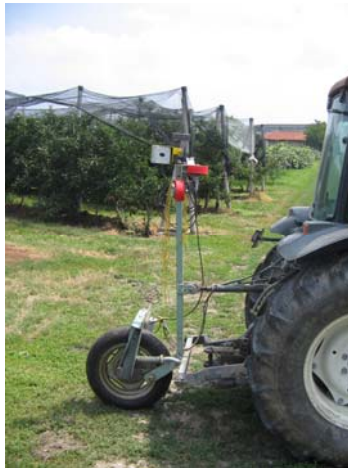
Figure 6. Device equipped with an ultrasonic sensor used in the tests.
