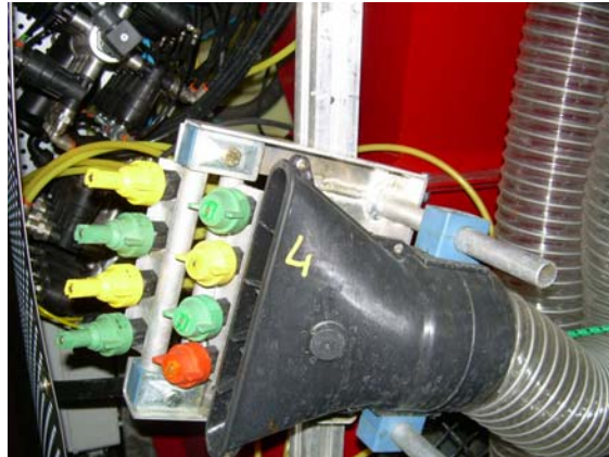
Figure 2. Detail of one single air spout equipped with conventional and air induction nozzles.
