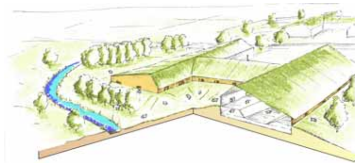
Fig Green roofed pig stables fitted carefully into the context of the landscape
