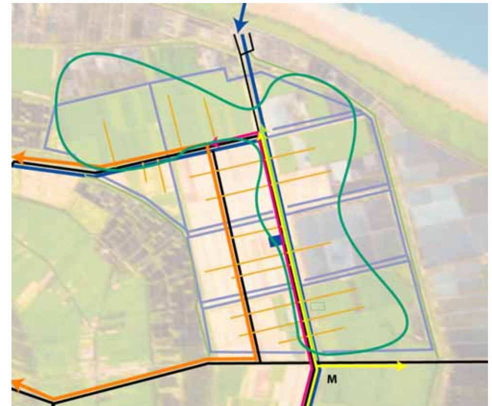
Fig internal transportation network The internal transportation network for all target groups links up to the outside world from the main entrance in the South, where roads and pedestrian routes begin and also the light rail starts. The westerly situated axis is mainly for cargo. The main roads follow the development axis, crossing at the central square. The road from the South is extended to the Yangtze River harbour in the North.
