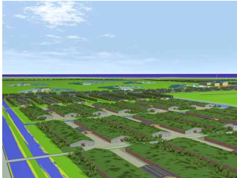
Fig profile F Multilayered Pig stables and Glasshouses The glass house complexes are single layered, double layered, being build on production units for mushrooms or on compost units. The production units for pigs are energy saving, two layered buildings, with green roofing, with innovative heat regulation
