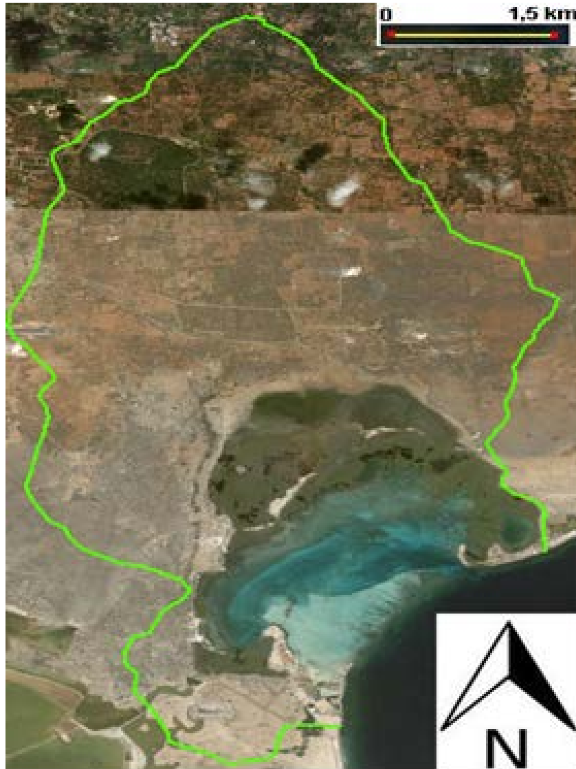
Fig. 4. Map of 22.6 km 2 Lac drainage basin showing the size of the catchment area.
