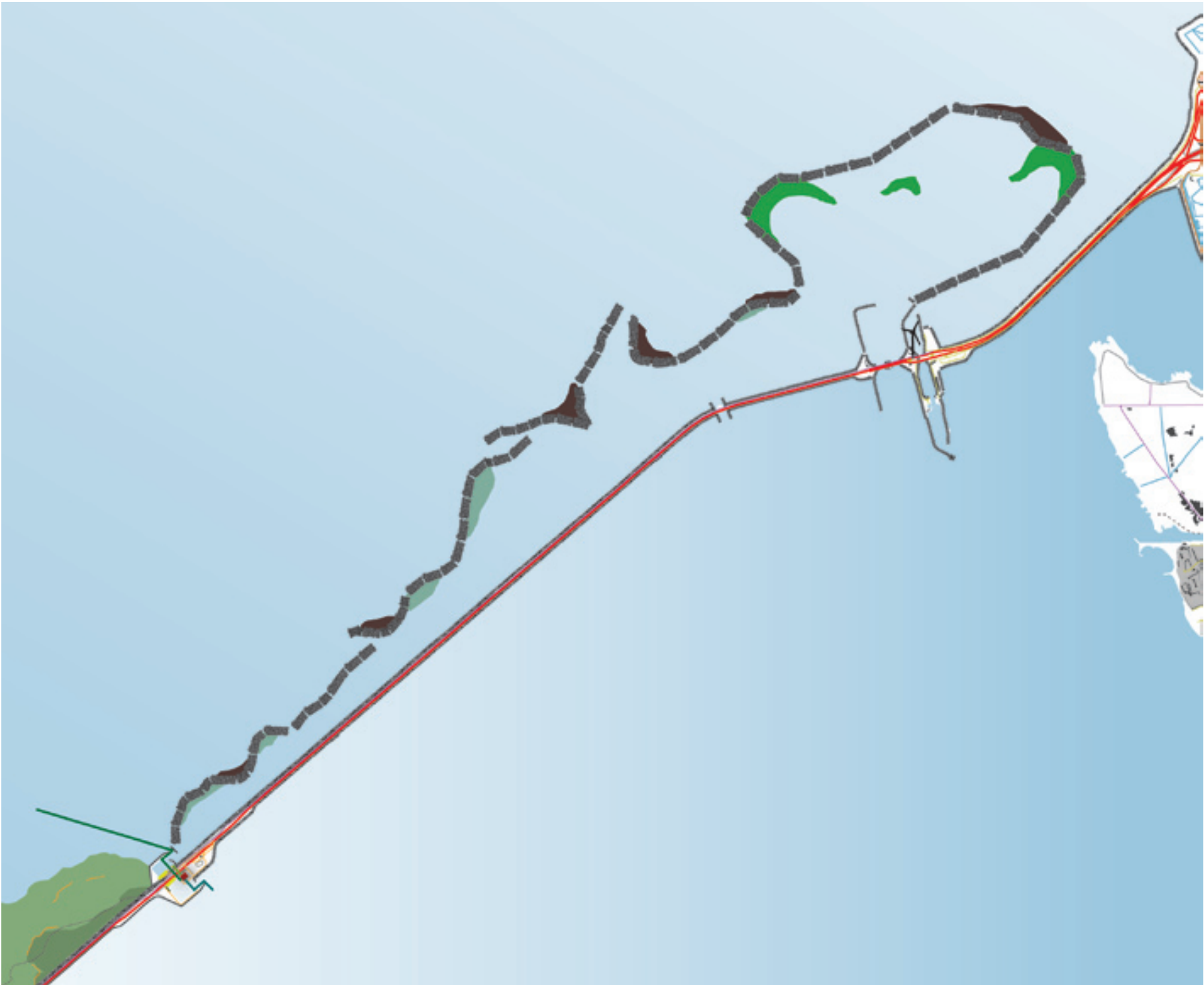
7.56. Design reefs at the side of the 'Waddenzee' to protect the dam against the fierceness of the waves and to lead the brackish water to the spouts.
