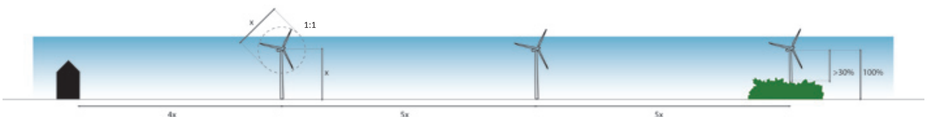
7.71. Design principles wind turbines. Step 2 results in a hub height of 80m and a distance in between turbines and houses (4 x 80 m) 320 m. 'The minimal distance between the turbines within a wind park is usually five times the rotor diameter' [Heersche J., 2006 -160]p225.
