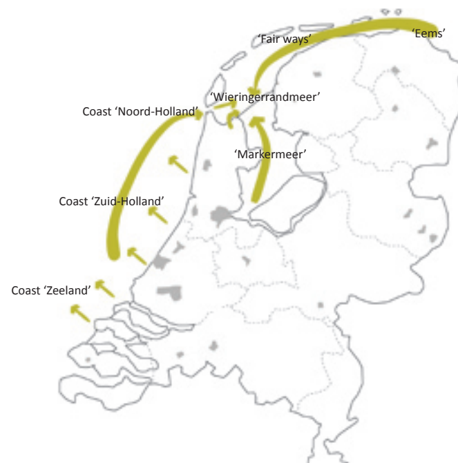
7.27. Materials like sand / silt from 'Markermeer', 'Wieringerrandmeer', fair ways and 'Eems' can be moved to 'De Afsluitdijk'. Because of the supspletion at the coast of the provinces 'Zeeland', 'Zuid-Holland' and 'Noord-Holland' will sand naturally move to the North
