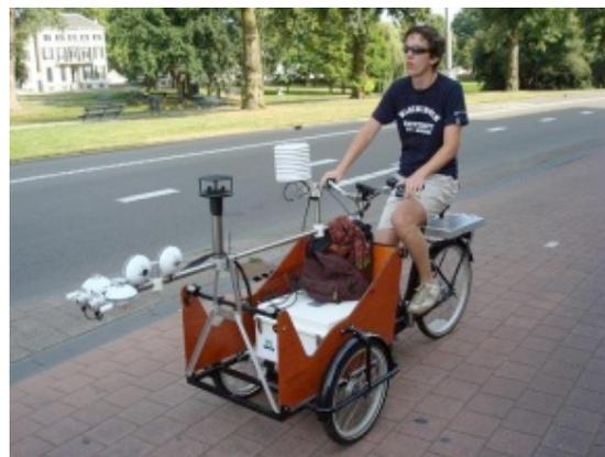
Fig 1: Instrumented tricycle (measuring temperature, humidity, wind speed, radiation components).
