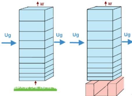
Fig 3: WRF 1D model set up: rural column (left), urban column (right).
