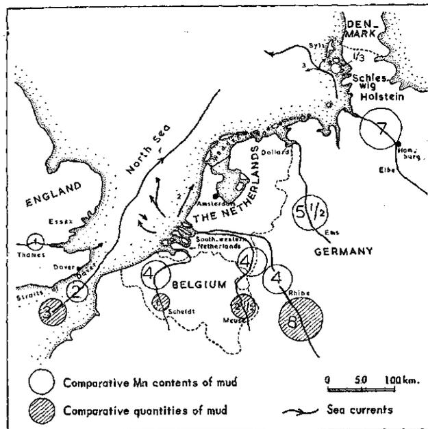
FIG. 3. Sources of mud and water movements in the North Sea area.
