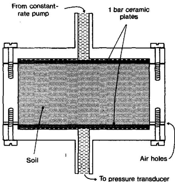
**Fig. 1—A cross-section of the soil cell. Soil diameter = 25.4 mm; soil depth = 12.9 mm.**
