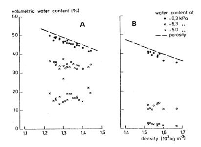
Fig. 8. Results of tension plate measurements on initially saturated samples from the soil layers 12.5-82.5 (A) and 97.5-160 (B) cm below surface, related to the dry bulk density of the samples
