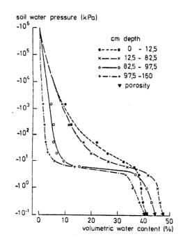
Fig. 9. Water retention curves derived from pressure cell and tension plate measurements on initially saturated soil samples from the experimental field
