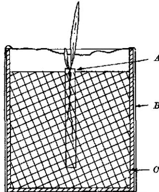
Fig. 1. Diagrammatic scheme of the apparatus. A, Root chamber; B, black plastic sheet to prevent growth of algae; C, glass pot with soil
