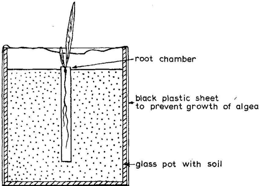
Fig. 1. Diagrammatic scheme of the experimental set up.
