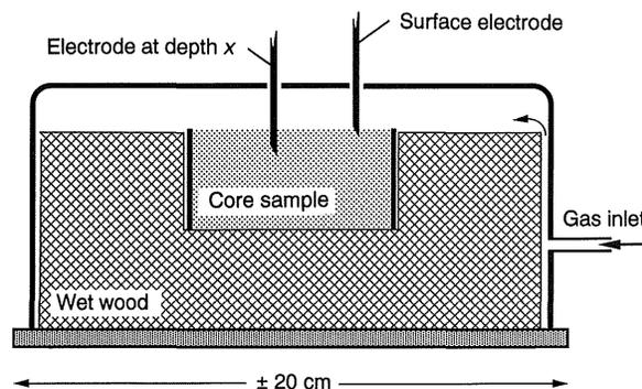
**Fig. 3.** A core sample placed in a box in which the oxygen concentration is periodically changed. Oxygen electrodes are placed in the soil and at the soil surface. The wet wood keeps the humidity high and reduces the box volume.
