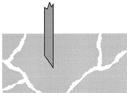
Fig. 1. An oxygen electrode penetrating the soil between air-filled macropores.
