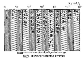
Fig. 2-Distribution constant ranges of elements in sewage sludge.
