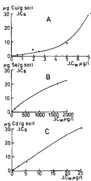
Fig. 3—Examples of adsorption isotherms found for the sandy loam soil using 0.0035M (CaCl<sub>2</sub> + NaCl + KCl) (3:2:2) as equilibrating solution.
