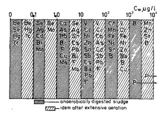
Fig. 1—Solution concentration ranges of elements in sewage sludge.
