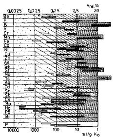
Fig. 4—Trace element mobility in a sandy top soil. White bars represent  $V_{\rm rel}$  or  $K_o$  found after equilibrating the soil with inorganic solution phases. Dark bars represent the range found after equilibrating with sewage sludge solution phases.
