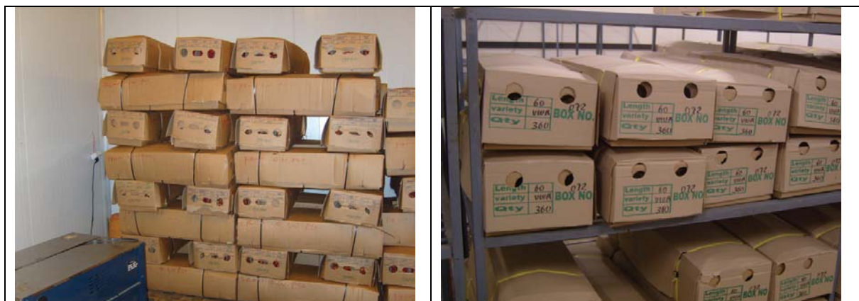
Figure 13.19: Loose stacking of boxes (left) or use of racks (right) allows more of the box surface to be exposed to cold air
