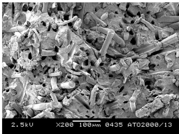
Figure 6.10. SEM micrograph of an uncompatibilised extrusion compound of 30 wt% flax/PP. Note the many deep holes where fibres have been pulled out.
