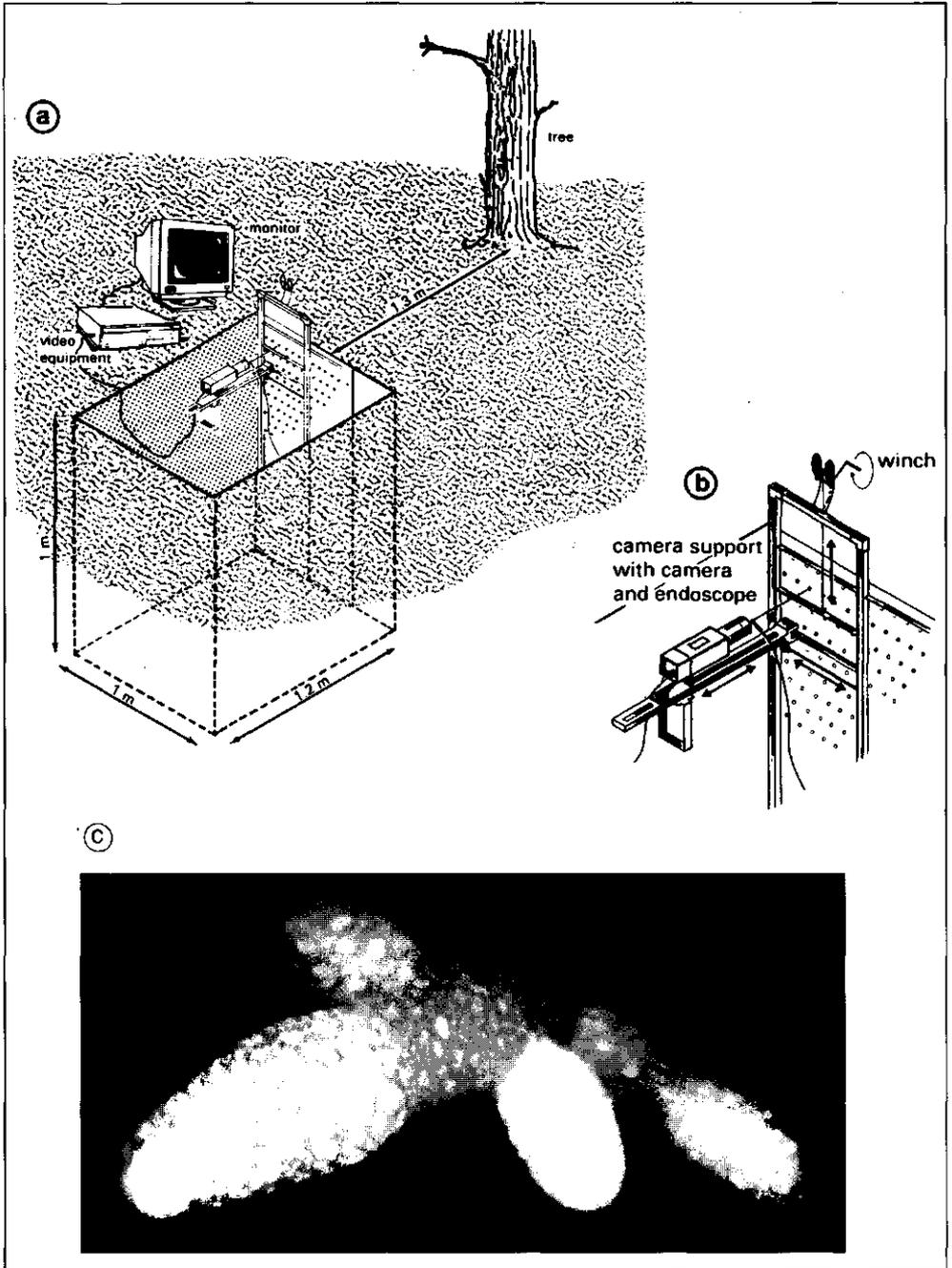
Figure 3.1. Schematic illustration of a) perforon root cellar with video equipment near a mature tree in a forest stand, b) camera stand with endoscope and CCD video camera and c) example of *Russula ochroleuca* mycorrhiza (diameter 1 mm) as visible in the perforon root cellar during development (endoscope photograph by G.M.J.H Ackermans).
