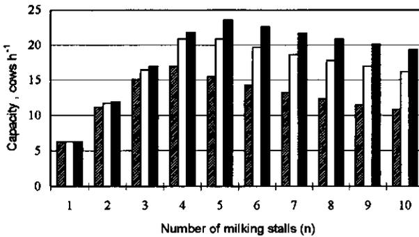
**Fig. 4.** The milking capacity (cows h<sup>-1</sup>) for an automatic milking system with 1 to 10 stalls in-line and for three different speeds of the robot wagon. 3 m min<sup>-1</sup> (shaded bar), 6 m min<sup>-1</sup> (white bar), 9 m min<sup>-1</sup> (black bar)
