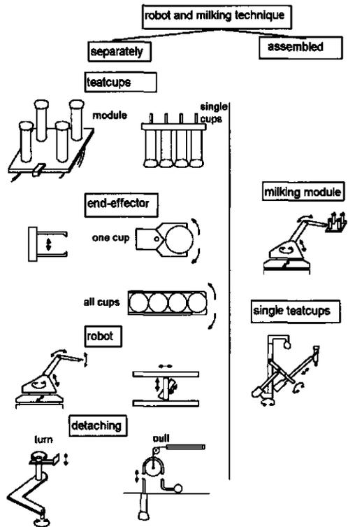
Fig. 2. An automatic milking system assembly
