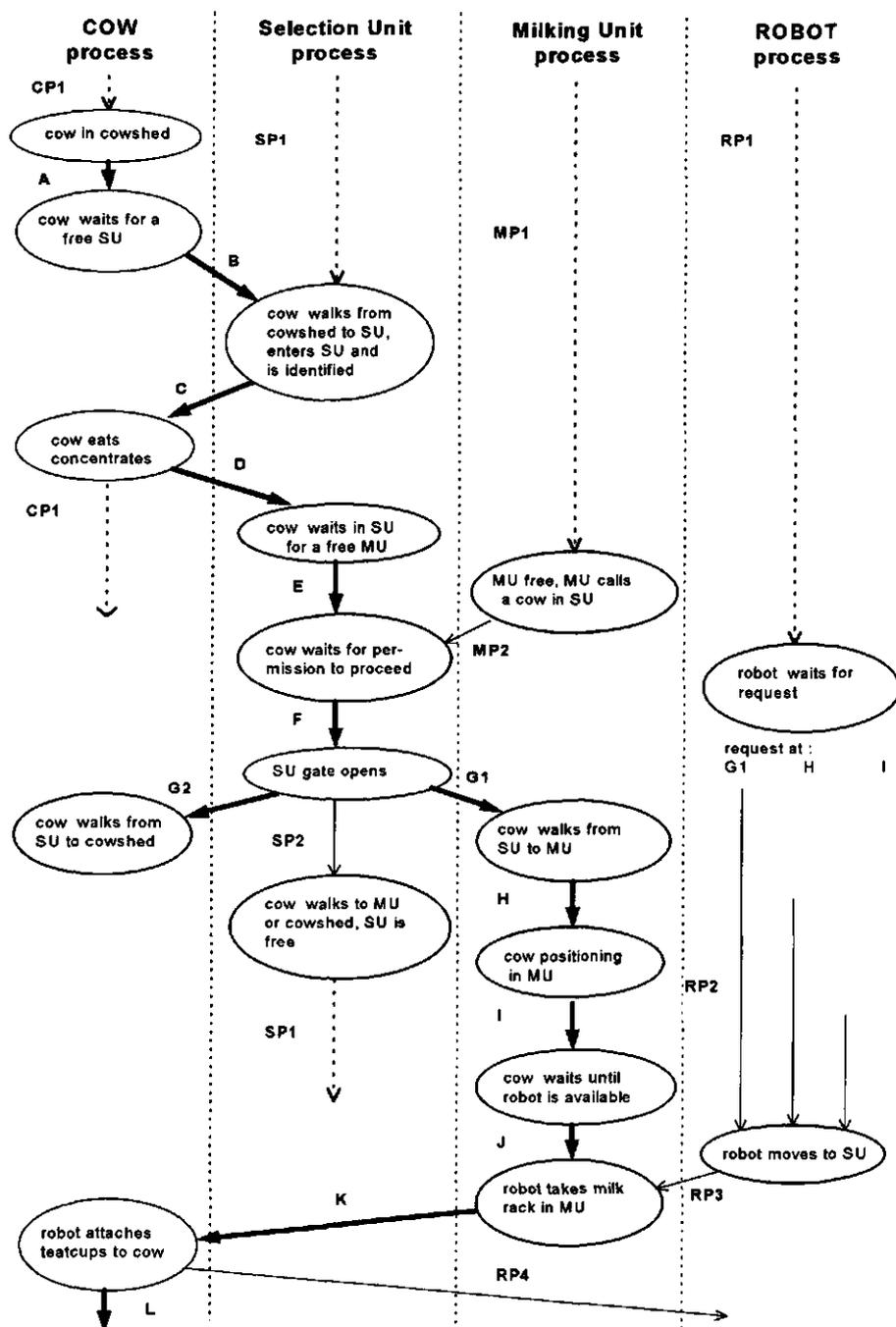
Fig. 5. Simplified schematic representation of the AMS simulation model showing COW, Selection Unit (SU), Milking Unit (MU) and ROBOT processes. To be continued
