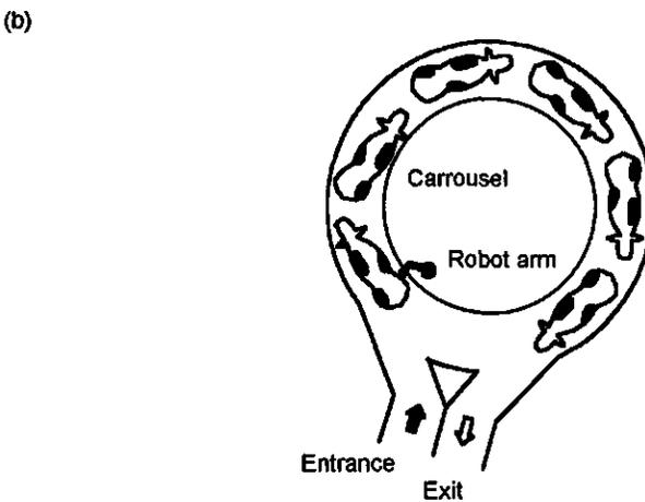
**Fig. 1.** Automatic milking system arrangements : (a) AMS with  $n$  milking stalls in-line or single tandem AMS arrangement; (b) Double tandem AMS arrangement; (c) Rotary tandem AMS arrangement
