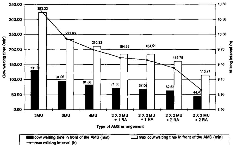
Fig. 10. The mean cow waiting time between presentation to SU and entering SU ('cow waiting for SU'), the mean and maximum cow waiting time between entering SU and the start of milking ('cow waiting for milking') and the maximum milking interval for different AMS arrangements. MU= milking unit; RA = robot arm
