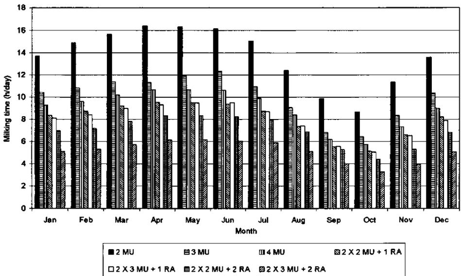
**Fig. 9.** Milking time (h/day) for automatic milking with human-controlled cow traffic and for different AMS arrangements. Herd size = 80 cows; Milking frequency = 3 times/day; MU = milking unit; RA = robot arm
