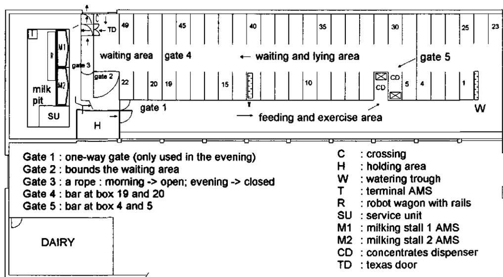
**Fig. 1.** Layout of the cubicle loose house with automatic milking system
