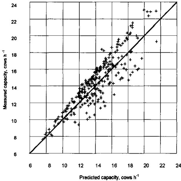
**Fig. 3.** Predicted capacities compared with measured capacities, calculated on the basis of one cycle. The full line indicates the ideal relation between the measured and predicted capacities
