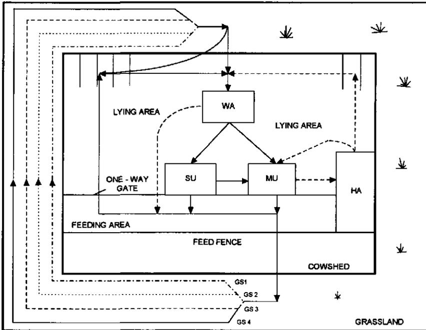
Fig. 3. Visual model of cow traffic with automatic milking in a total farm system, used as basis for a task-time program for automatic milking; MU = milking unit; SU = cow selection unit; WA = waiting area; HA = holding area; GS1...2 = grazing systems; GS1 = unrestricted grazing; GS2 = restricted grazing during one long period; GS3 = restricted grazing during one short period; GS4 = restricted grazing during two short periods
