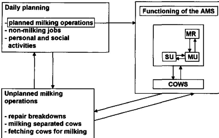
**Fig. 4.** Interrelations between the planned and unplanned operations and jobs of the farmer and the functioning of the automatic milking system (AMS = automatic milking system; SU = selection unit; MU = milking unit; MR = milking robot)
