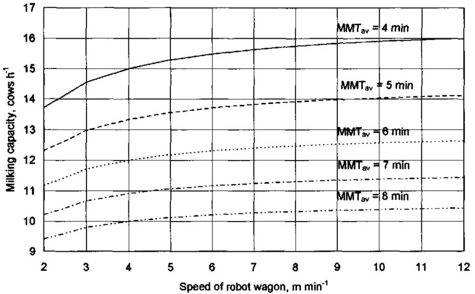
Fig. 6. The milking capacity (cows  $h^{-1}$ ) as a function of the speed of the robot wagon with different average machine milking times ( $MMT_{av}$ ) and for a two-stall automatic milking system
