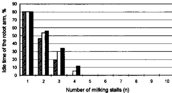
**Fig. 5.** The idle time of the robot arm (as percentage of the total process time) for an automatic milking system with 1 to 10 stalls in-line and for three different speeds of the robot wagon. 3 m min<sup>-1</sup> (shaded bar), 6 m min<sup>-1</sup> (white bar), 9 m min<sup>-1</sup> (black bar)
