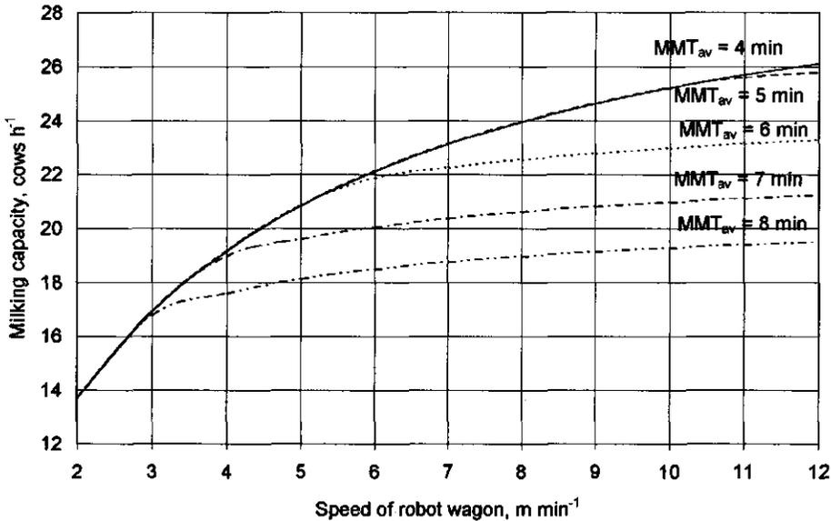
Fig. 8. The milking capacity (cows  $h^{-1}$ ) as a function of the speed of the robot wagon with different average machine milking times ( $MMT_{av}$ ) and for a four-stall automatic milking system
