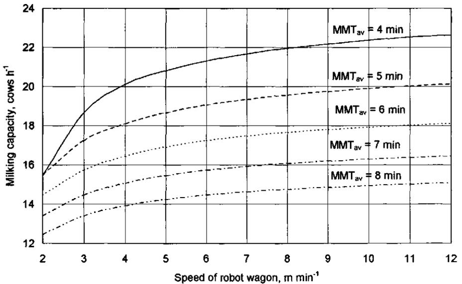
Fig. 7. The milking capacity (cows  $h^{-1}$ ) as a function of the speed of the robot wagon with different average machine milking times ( $MMT_{av}$ ) and for a three-stall automatic milking system
