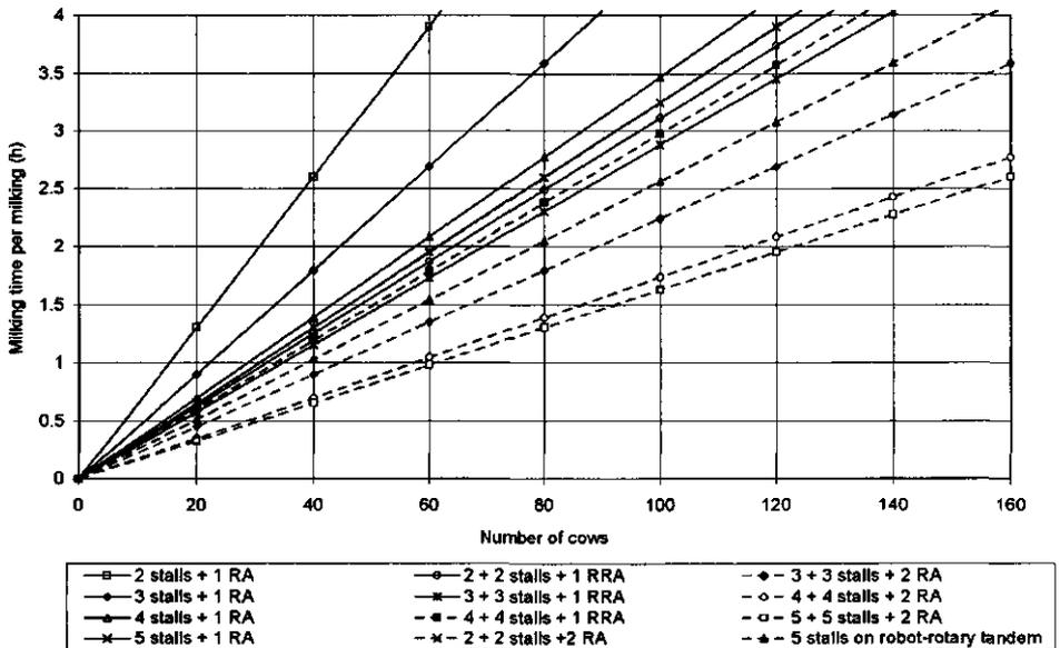
**Fig. 1.** The milking time per milking for different herd sizes, a milking frequency of three times a day and with the AM-HCT method. The formula of tuning to determine the milking capacity has been used under improved working conditions of the milking robot. RA = robot arm; RRA = rotary robot arm
