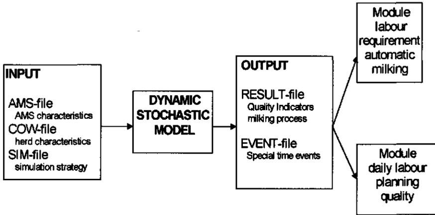
**Fig. 1.** Schematic overview of the modelling approach. Information flow between the models is indicated by arrows. Use of the modules is optional
