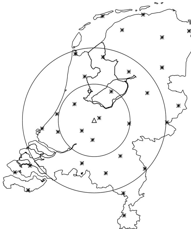
**Fig. 9.** The locations of the KNMI radar site (Δ) and the automatic KNMI rain gauges (\*) in The Netherlands. Concentric circles around the radar antenna with a radius of 50 and 100 km give an indication of the distance of the gauges to the radar site.
