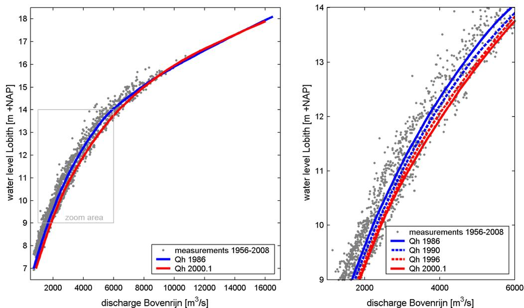
Figure 1. Different rating curves (Qh 1986, 1990, 1996 and 2000.1) together with the discharge measurements from 1956 - 2008 show the temporal change of the stage-discharge relation of Lobith
