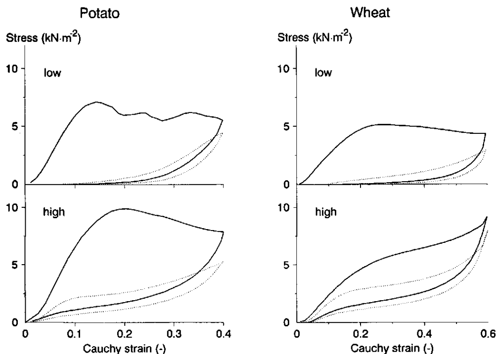
Figure 5.11 Stress-strain curves of potato and wheat starch breads that had been compressed and decompressed twice. The initial strain rates of compression were 1.7 \times 10^3 \text{ s}^{-1} (low) and 1.7 \times 10^1 \text{ s}^{-1} (high). The solid line shows the first compression and de-compression and the dashed line the second ones. The starch breads had been stored for 1 day at 20^\circ \text{C} .
