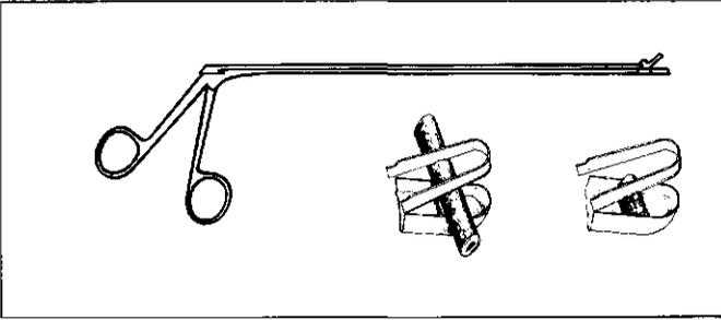
Figure 43 : Biopsy forceps as used in Wageningen to remove selected parts of the fine roots that grow through the perforations. After the a piece of the root, for instance an ectomycorrhizal root tip, has been cut of, the piece remains relatively clean inside the small chamber
