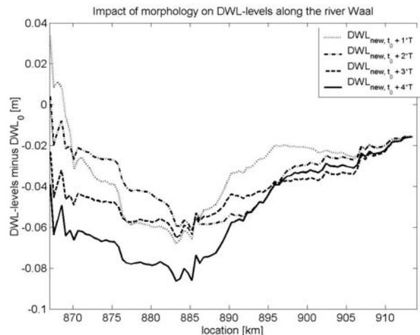
Figure 9. Impact of morphology of DWL-levels along the river Waal: change in DWL level with respect to  $DWL_0$ .
