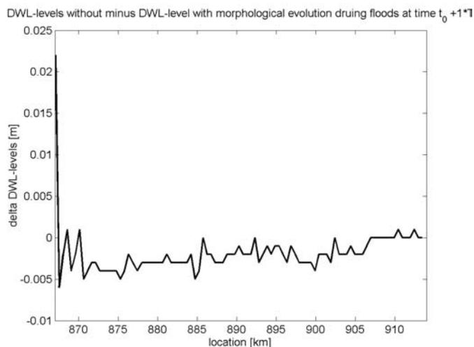
Figure 14. Impact of morphological changes during flood circumstances: difference between DWL levels if morphological changes during floods are neglected and considered.
