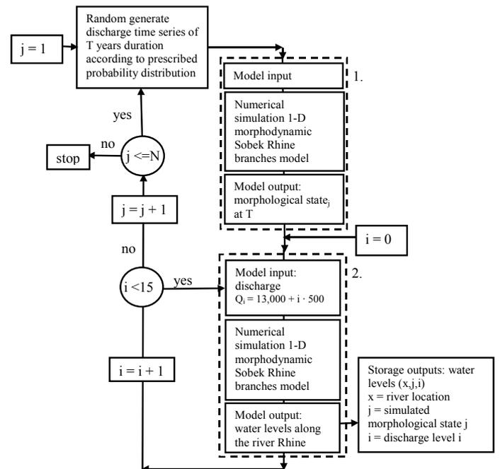
Figure 7. Design water levels: computation method with the random variables: discharge and bed level.
