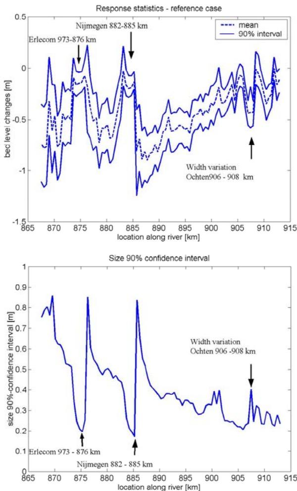
Figure 4. Spatial variation of statistical properties of the bed level change after 100 years in the Waal section between Pannerdendse Kop (km 886) and Tiel (km 915).
