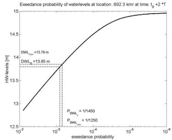
Figure 8. Exceedance probability of water levels at location 892.3 km at time  $t_0 + 2 \cdot T$  for Case 1.
