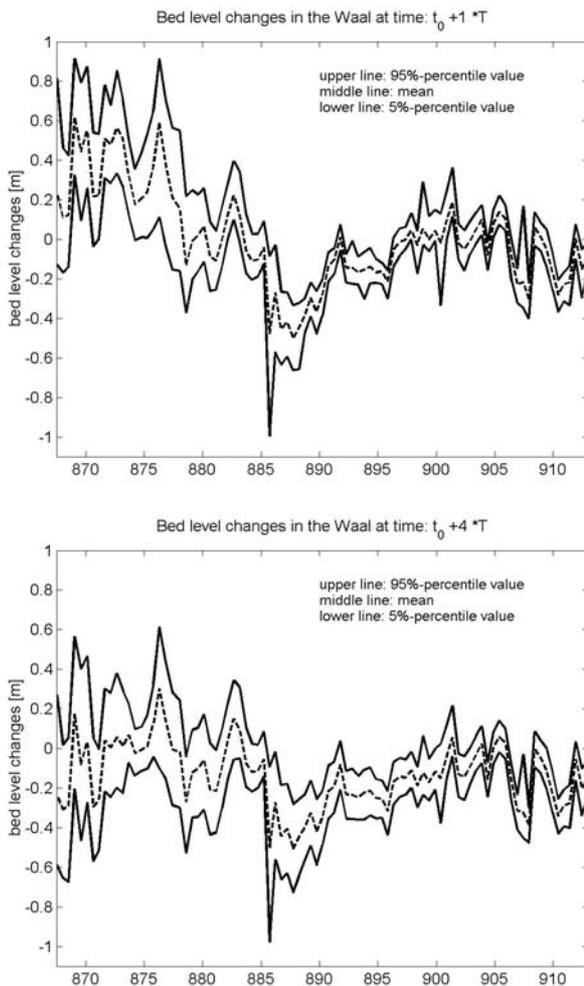
Figure 11. Spatial variation of the statistical properties of the morphological response in the Waal at time  $t_0 + T$  and  $t_0 + 4 \cdot T$ .
