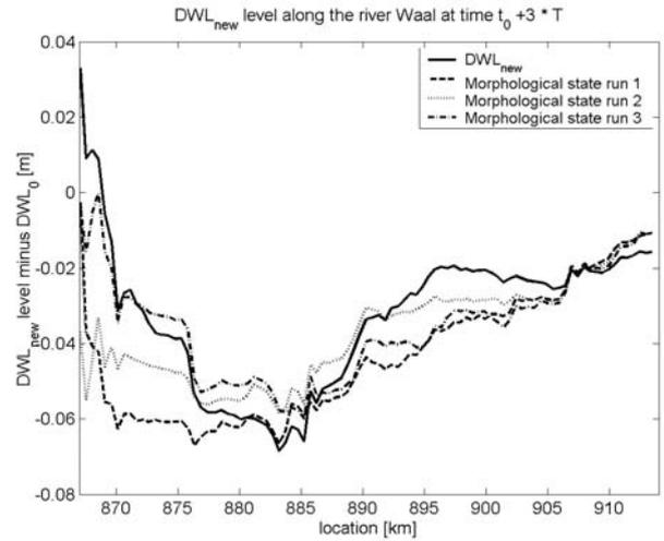
Figure 12. Impact of morphology of  $DWL$ -levels along the river Waal: change in  $DWL_{new}$  levels and  $DWL$  levels of single morphological simulations with respect to  $DWL_0$ .
