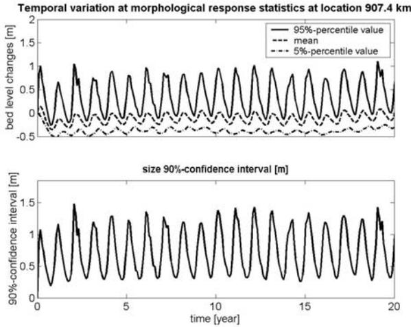
Figure 6. Temporal variation of statistical properties of the bed level change in the Waal at location 907.4 km in the Willem-sploder.
